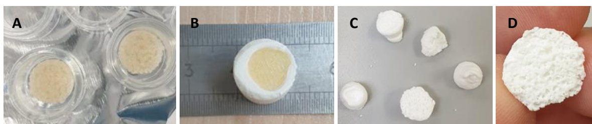
Figure 4-8: Stages of incorporating 3D printed hexagonal part (Figure 4-1 D) into AW2 TIPS. A) The 3D printed hexagonal pattern was placed at the bottom of the glass mould, and then AW2 slurry poured on top. B) the bottom of freeze-dried TIPS AW2 PLA green part with the 3D printed part incorporated. C) multiple sintered AW2 scaffolds that had the hexagonal 3D printed part incorporated. D) magnified image of bottom of AW2 scaffold after sintering, showing the pores caused by the 3D printed part.
