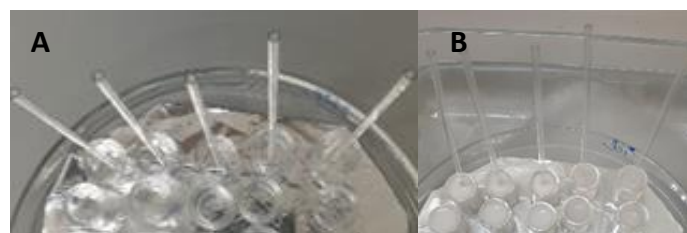
Figure 4-5: Process of slurry addition to glass tube/channel in glass moulds. A) Glass tubes are superglued to the middle of the glass moulds. B) slurry containing AW2 poured into glass moulds.
