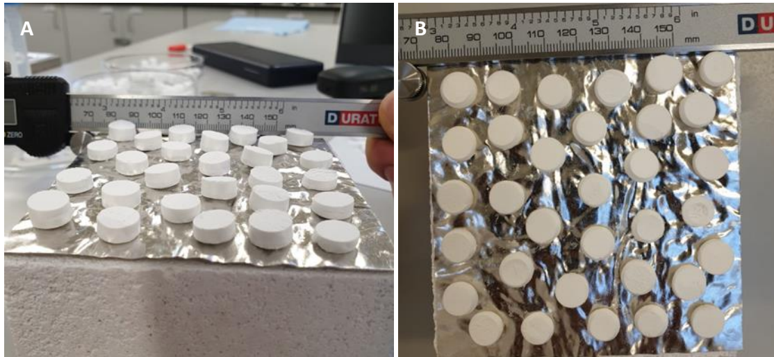
Figure 4-4: Porous AW2 scaffolds post sintering. A) Scaffolds cut to approximately 3-4 mm height. B) Scaffolds from a top view.
