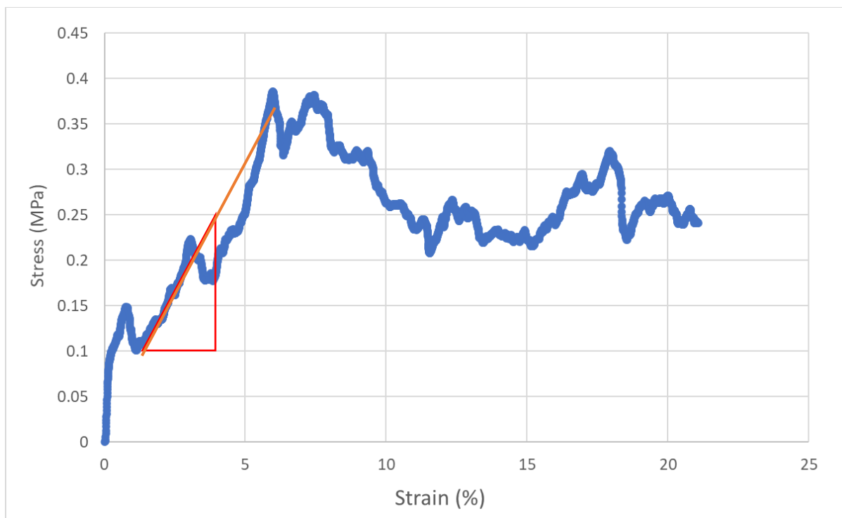
Figure 5-32: A stress - strain graph of a modified AW2 scaffold seeded with osteoblast cells for 21 days.
