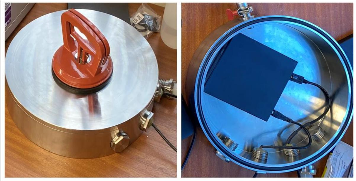
Figure 3-5 cylindrical vacuum chamber (left), the DVD Lightscribe writer in the vacuum chamber (right).
