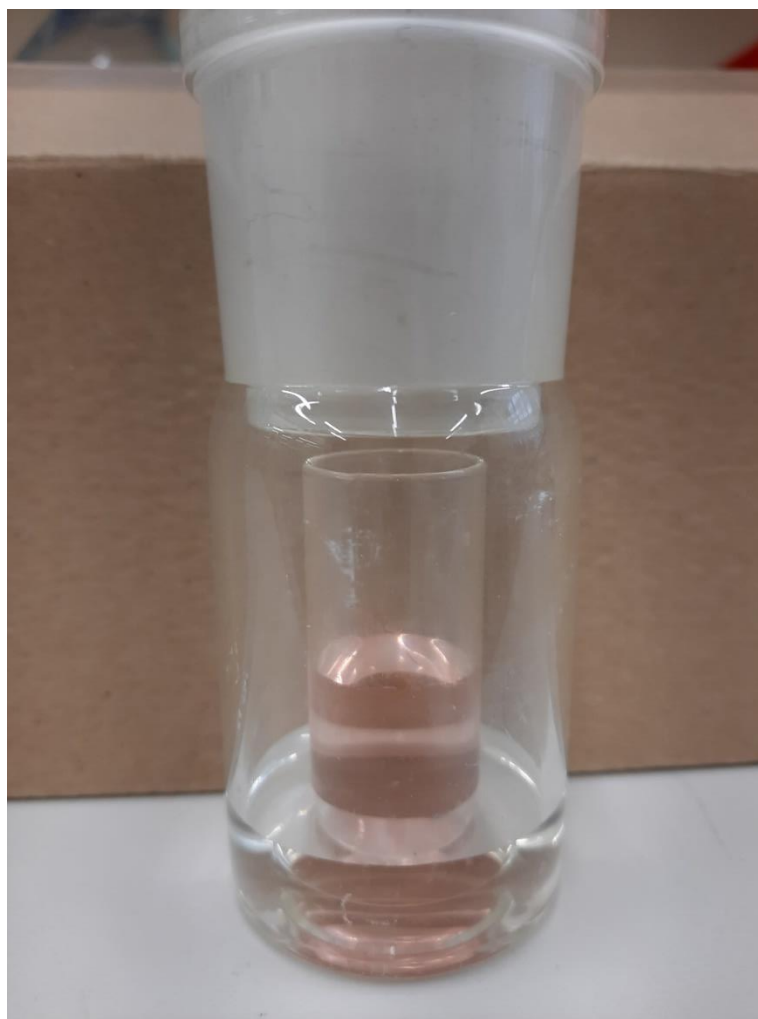
Figure 3.28. Example of a vapour diffusion crystallisation, the outside chamber contains diethyl ether which will diffuse into the inner chamber containing a methanol solution of a cobalt metal complex.
