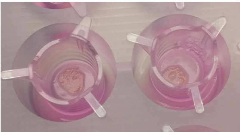
Figure 8-3: Tissue samples with printed gels on to. Left shows a 4 layer single droplet gel and right shows a 4 layer 2x2 gel
