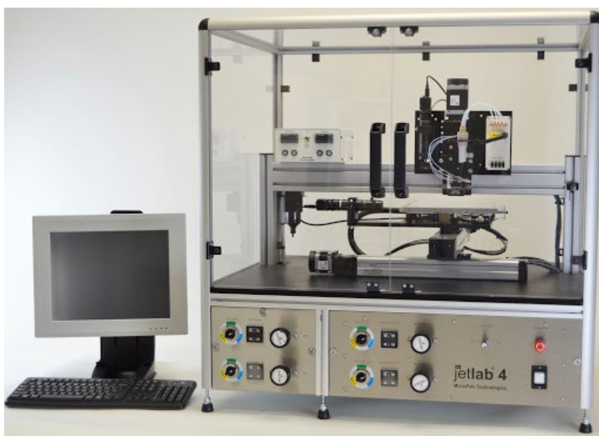
Figure 3-3: JetLab® 4 XL (MicroFab, USA) printing work station combined with the JetDrive® printer drive electronics unit
