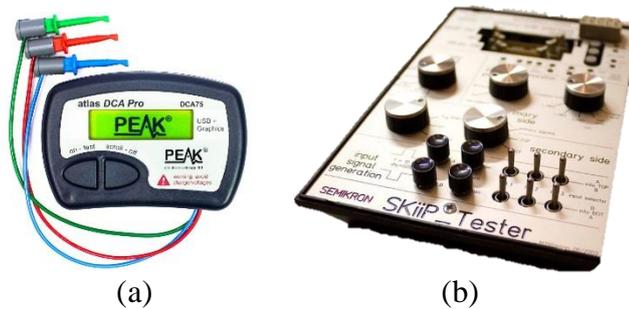
**Figure 5.1 (a) DCA75 (Atlas DCA Pro) from Peak Electronics, (b) SKiiP tester developed and produced by Ing. Büro M.Billmann.**
