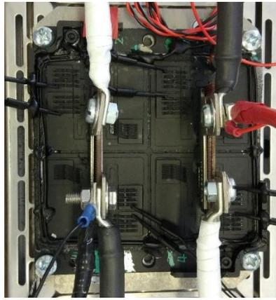
**Figure C. 22 The Dynex module under test.**
