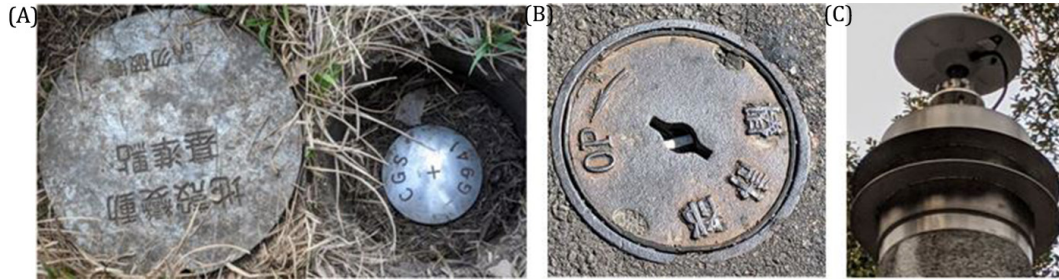
Figure 4.2: (A) Levelling and (B) geodetic benchmark in Taichung city, Taiwan and (C) a GPS antenna in Puli City, Taiwan. [Photo credit: Marine Roger]
