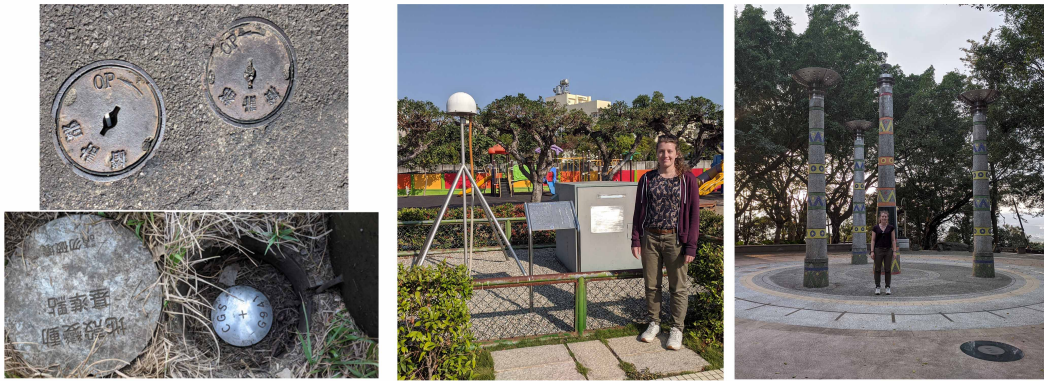
Figure 7.7: (left) Two benchmarks and a levelling reference. (middle) A continuous GNSS station in Wuguang Elementary School. (right) Continuous GNSS station.
