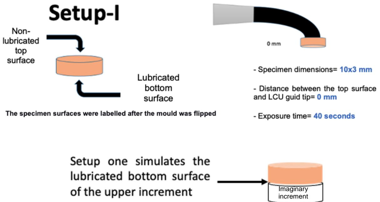
**Figure 5-14:** Setup one, showing the degree of conversion and Martens hardness tests on the specimen top non-lubricated surface and bottom lubricated surface
