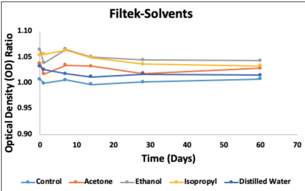
Figure 5-24: Optical density ratio of solvents over time for Filtek
