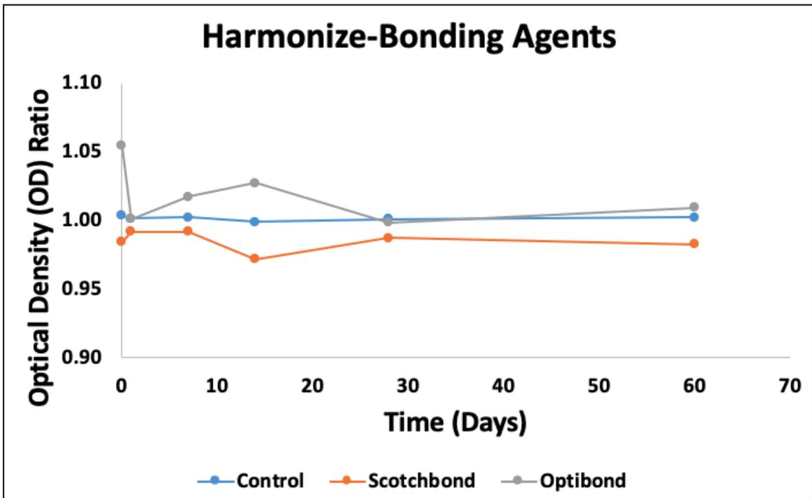
Figure 5-27: Optical density ratio of bonding agents over time for Harmonize
