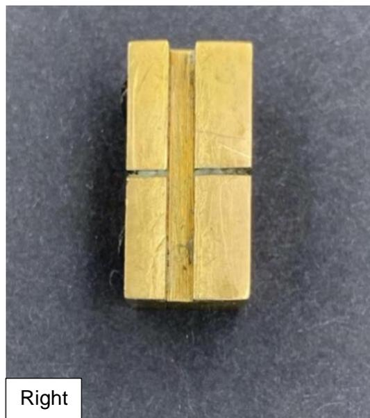
**Figure 5-2:** Left: Separated mould parts; Right: Assembled mould and a view of the mould slot
