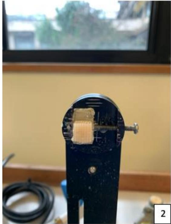
Block attached to the saw arm to begin sectioning
