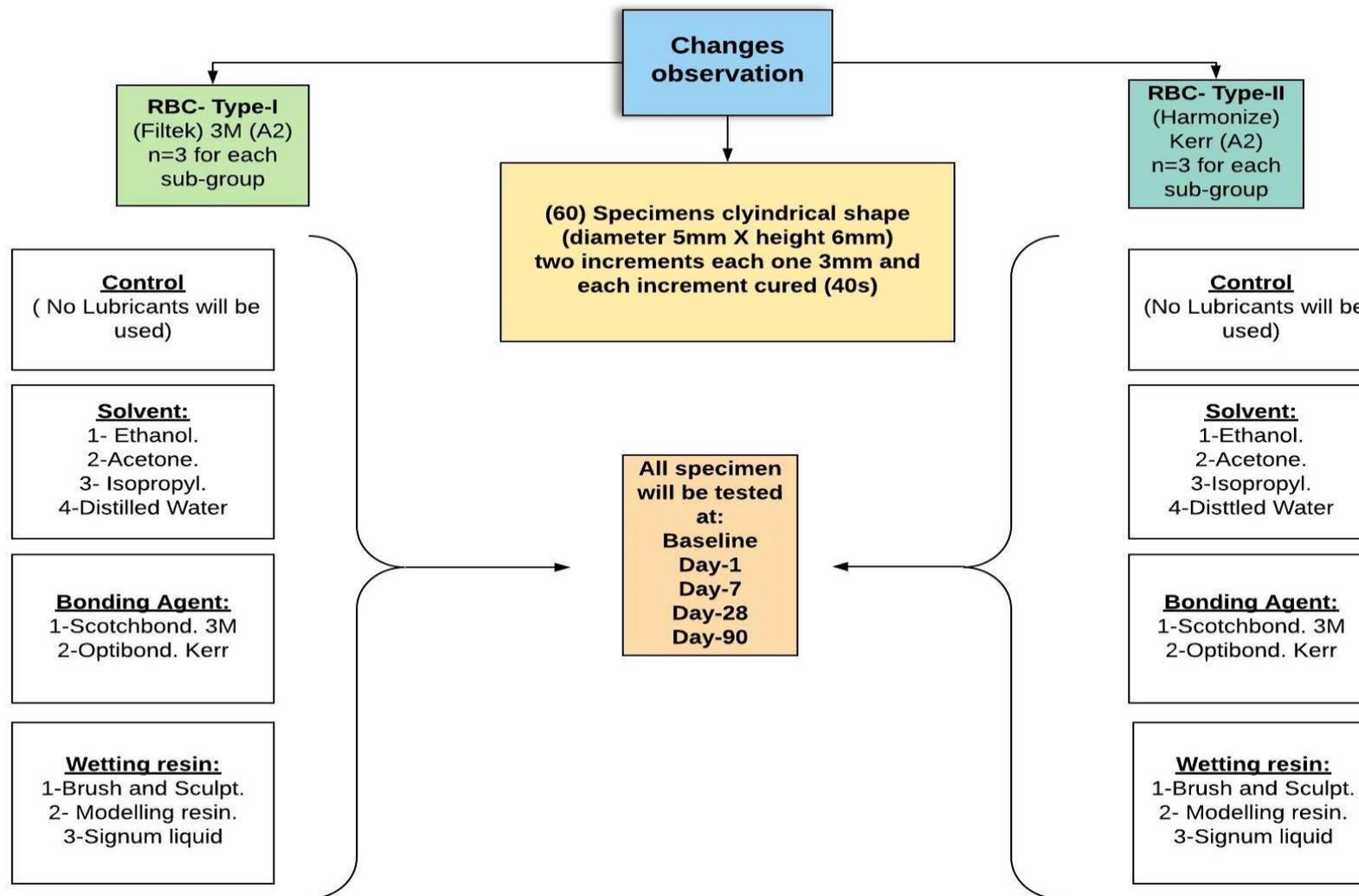
**Figure 5-6:** Specimen dimensions and key data for the observation of changes at the interface between the increments Specimen dimensions and key data for the observation of changes at the interface between the increments
