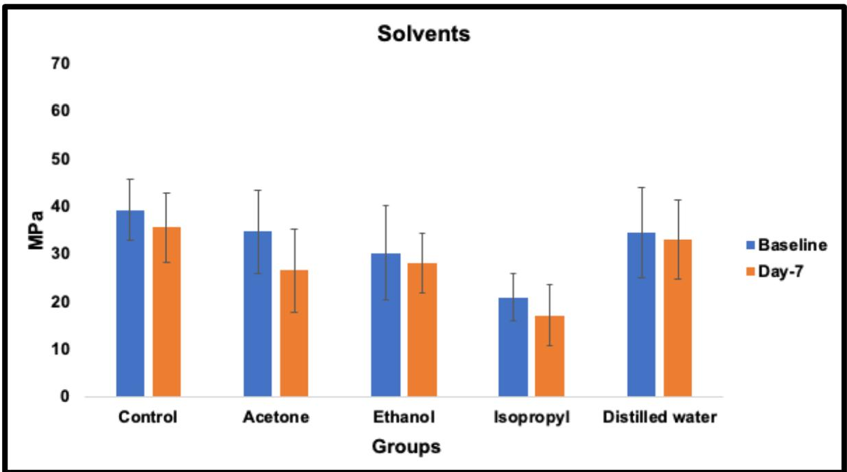
**Figure 6-9:** Mean and standard deviation values for the microtensile strength of Filtek RBC treated with solvents as ILs
