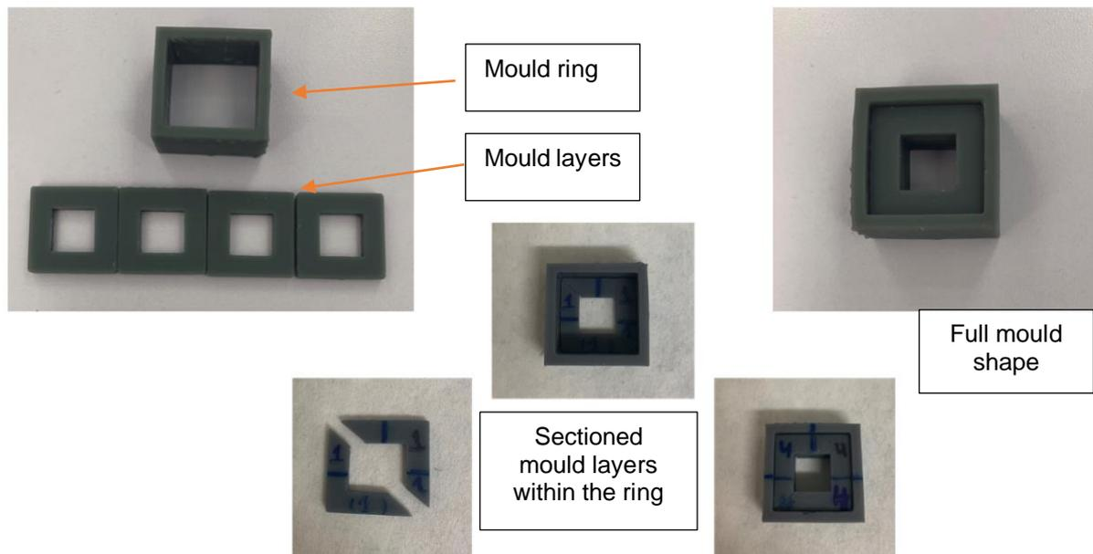
**Figure 6-1:** The final shape of the mould's layers and holding ring
