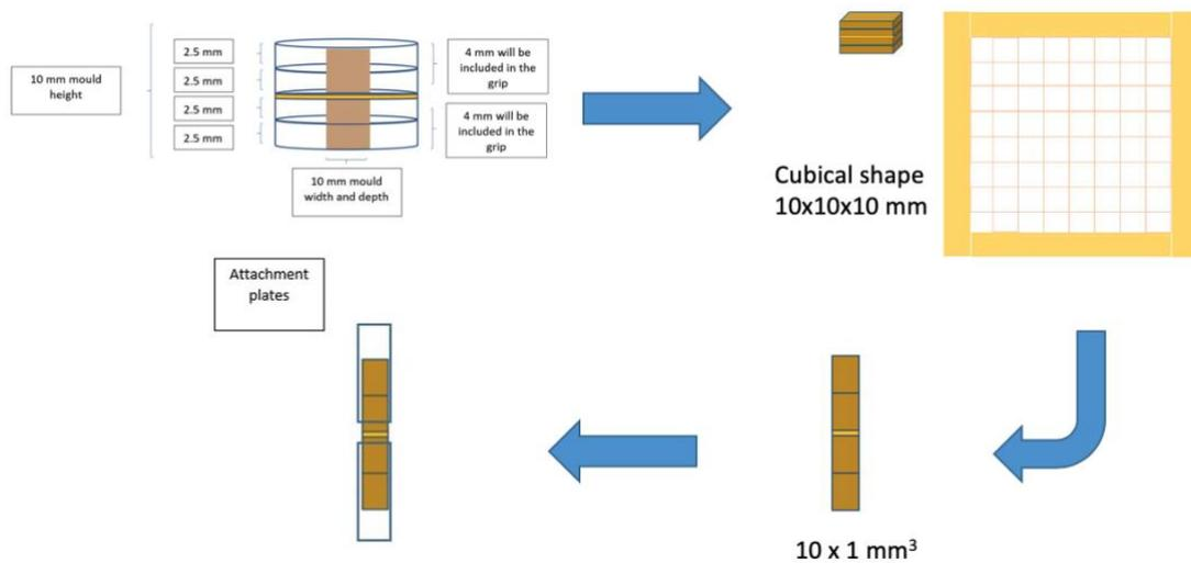
**Figure 6-2:** The design and preparation process for producing the blocks and specimens for the microtensile test
