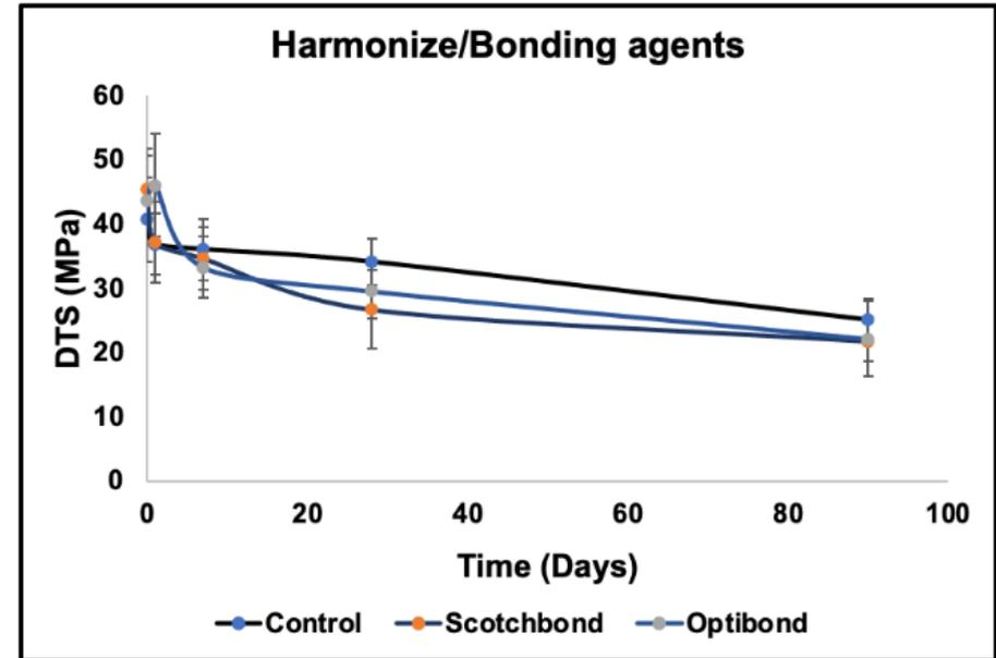
**Figure 5-48:** Bonding agent group mean (MPa) and standard deviation DTS for Filtek and Harmonize, stored in distilled water <90 days
