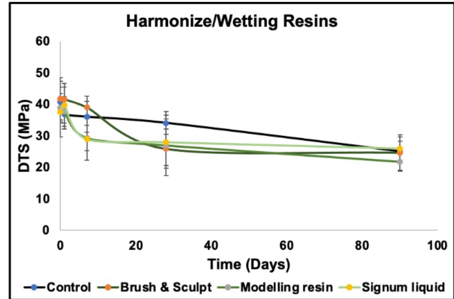
**Figure 5-49:** Wetting resin group mean (MPa) DTS and standard deviation values for Filtek and Harmonize, stored in distilled water <90 days
