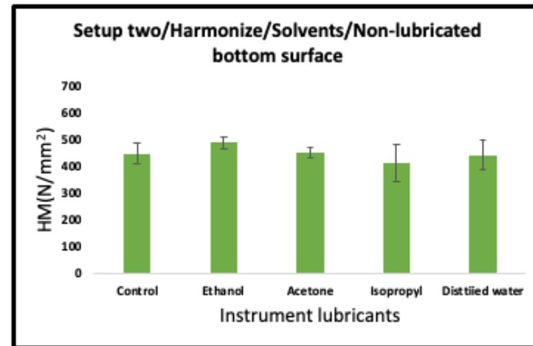
**Figure 5-41:** Mean and standard deviation values for Martens hardness tests (Filtek & Harmonize) for solvent-lubricated top surface and non-lubricated bottom surface in setup two
