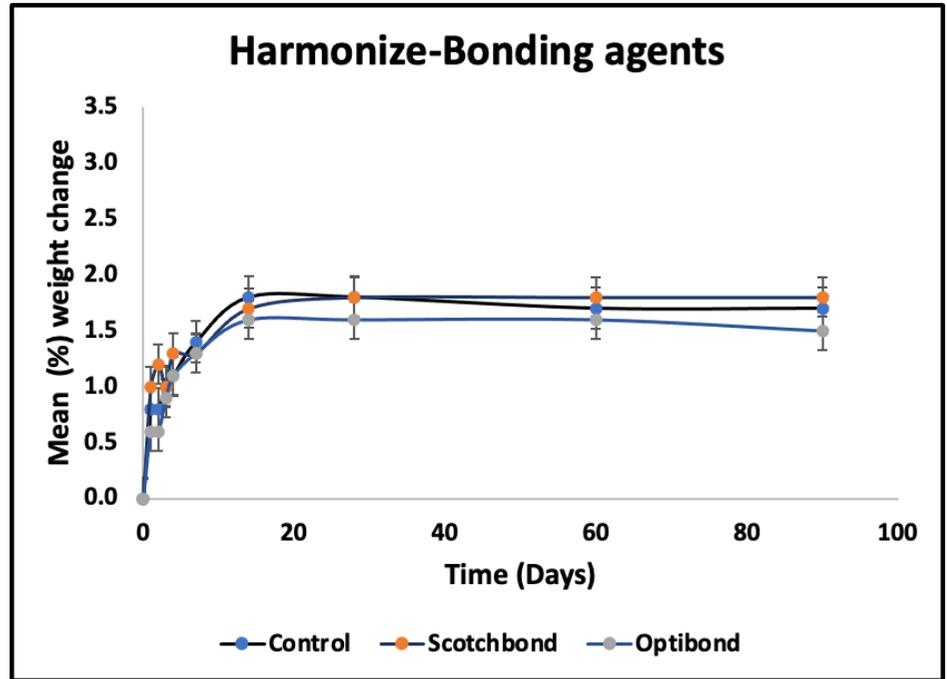
**Figure 5-45:** Bonding agent group means of % weight change and standard deviation for the water uptake in Filtek and Harmonize, stored in distilled water <90 days
