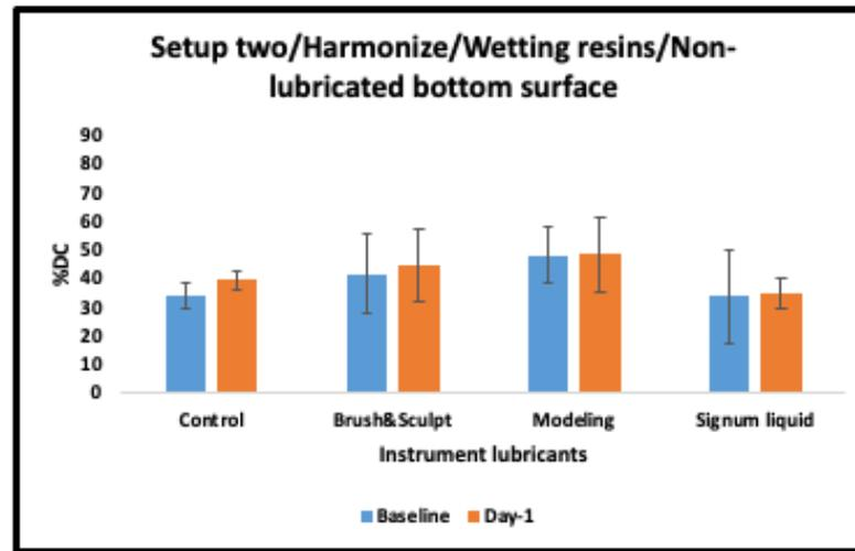
**Figure 5-37:** Mean and standard deviation values for the degree of conversion for Filtek and Harmonize for wetting resins-lubricated top surface and non-lubricated bottom surface/setup two
