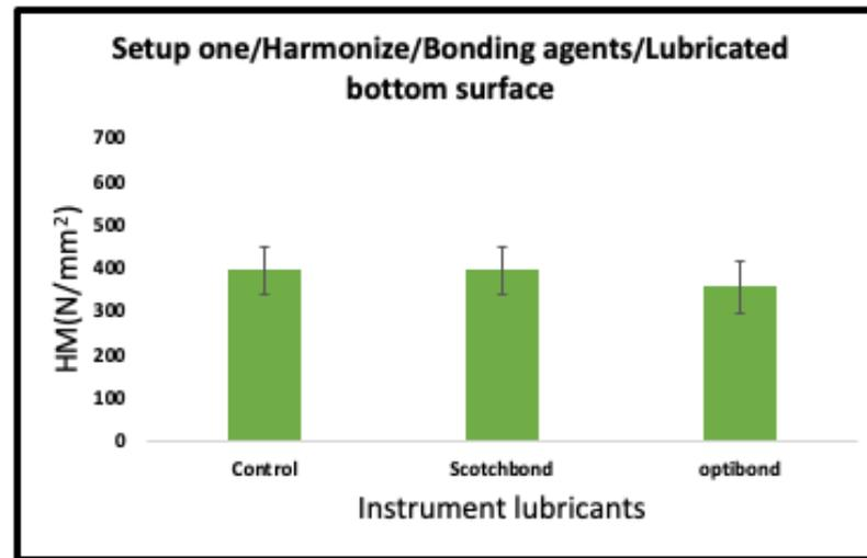
**Figure 5-39:** Mean and standard deviation values for Martens hardness tests (Filtek & Harmonize) for non-lubricated top surface and bonding agent-lubricated bottom surface in setup one
