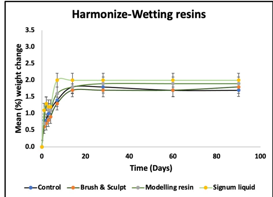
**Figure 5-46:** Wetting resin group mean % weight change and standard deviation of water uptake for Filtek and Harmonize, stored in distilled water <90 days
