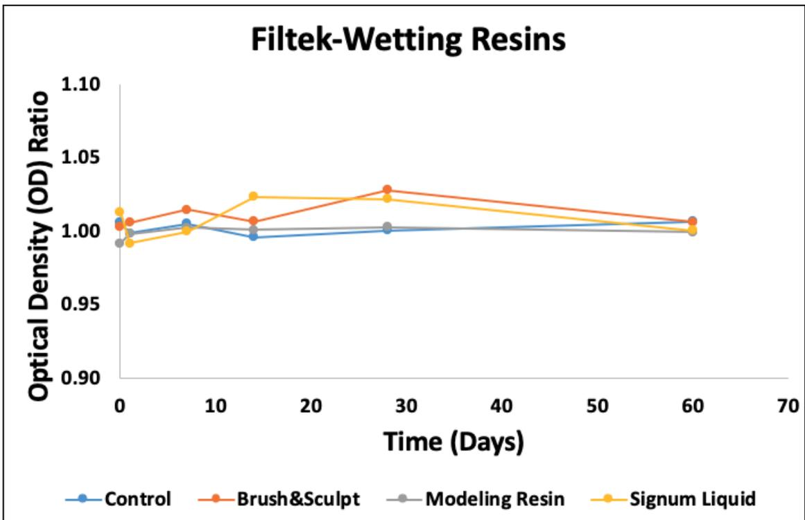
Figure 5-28: Optical density ratio of wetting resins over time for Filtek and Harmonize
