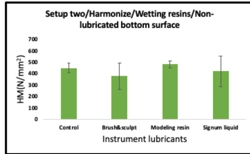
**Figure 5-43:** Mean and standard deviation values for Martens hardness tests (Filtek & Harmonize) for wetting resin-lubricated top surface and non-lubricated bottom surface in setup two
