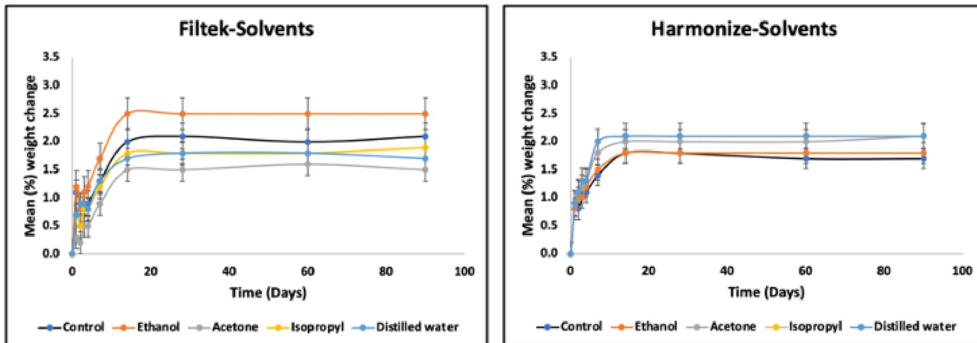
**Figure 5-44:** Solvent group % means for weight change and standard deviation for water uptake for Filtek and Harmonize stored in distilled water <90 days
