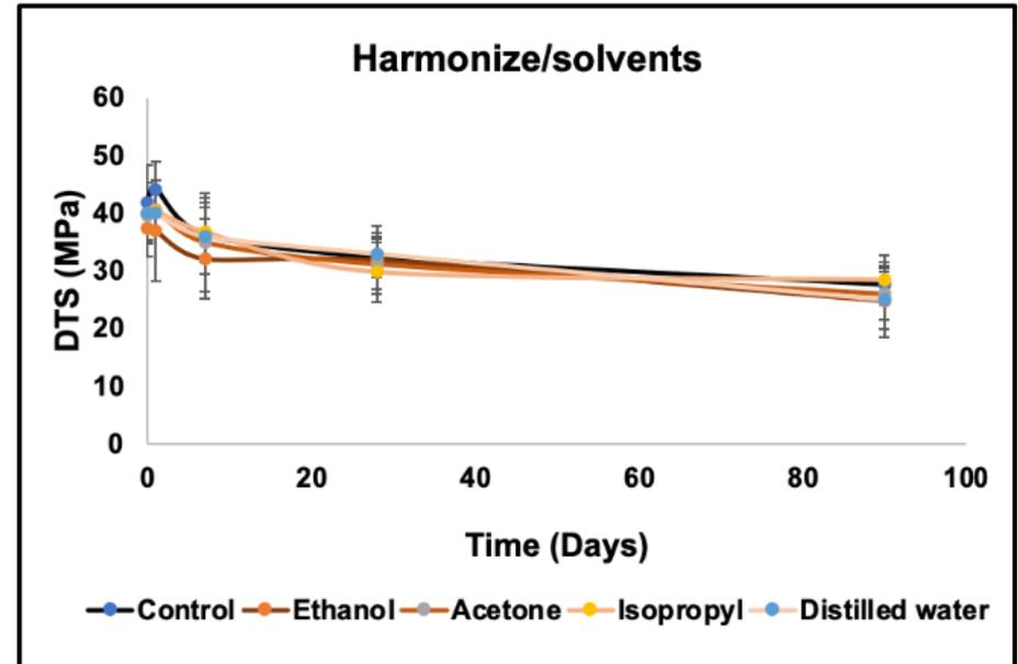
**Figure 5-47:** Solvents groups mean (MPa) DTS and standard deviation values for Filtek and Harmonize, stored in distilled water <90 days
