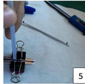
check and standardise 4 mm reference points on both attachment parts
