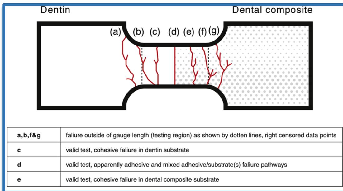
**Figure 2-22:** Fracture failures in specimens by location taken from (Armstrong *et al.*, 2017)
