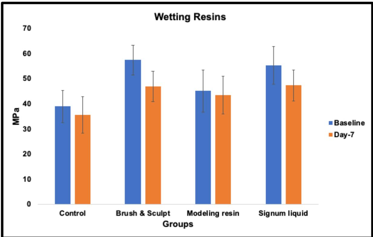
**Figure 6-11:** Mean and standard deviation values for the microtensile strength of Filtek RBC treated with wetting resins as ILs
