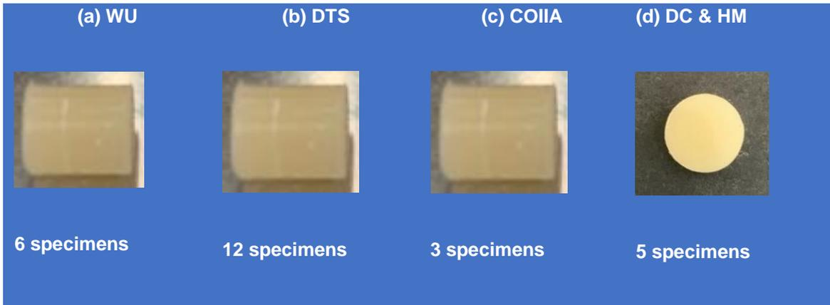
**Figure 5-10:** Final specimen shapes and number for each experiment
