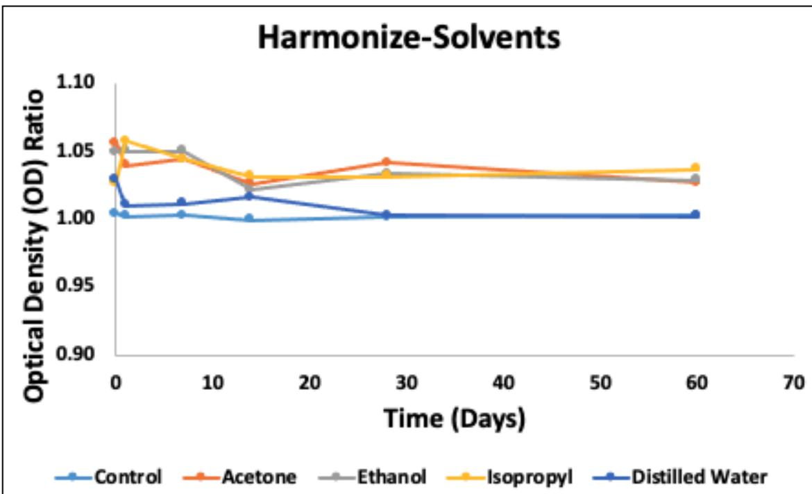
Figure 5-25: Optical density ratio of solvents over time for Harmonize
