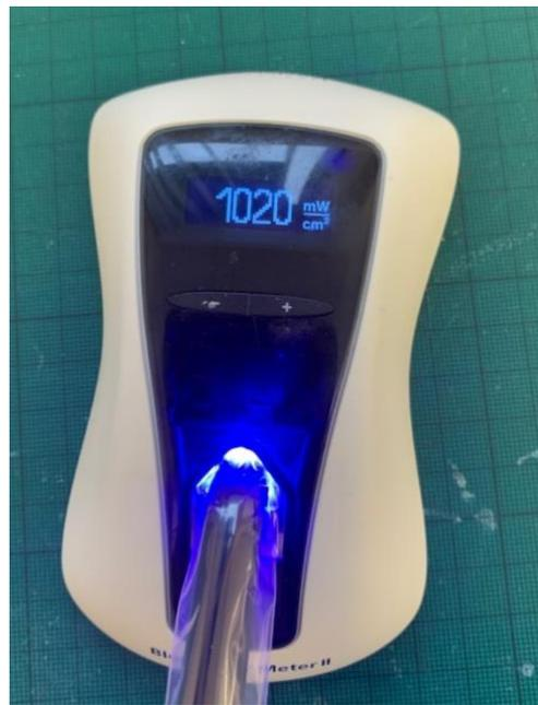
**Figure 5-1:** Bluephase Meter II and irradiance measuring of the LED LCU
