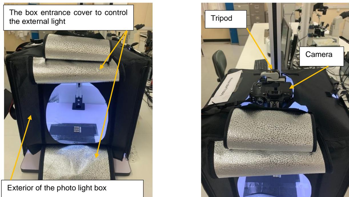
**Figure 5-17:** The exterior of the professional photo light box and tripod
