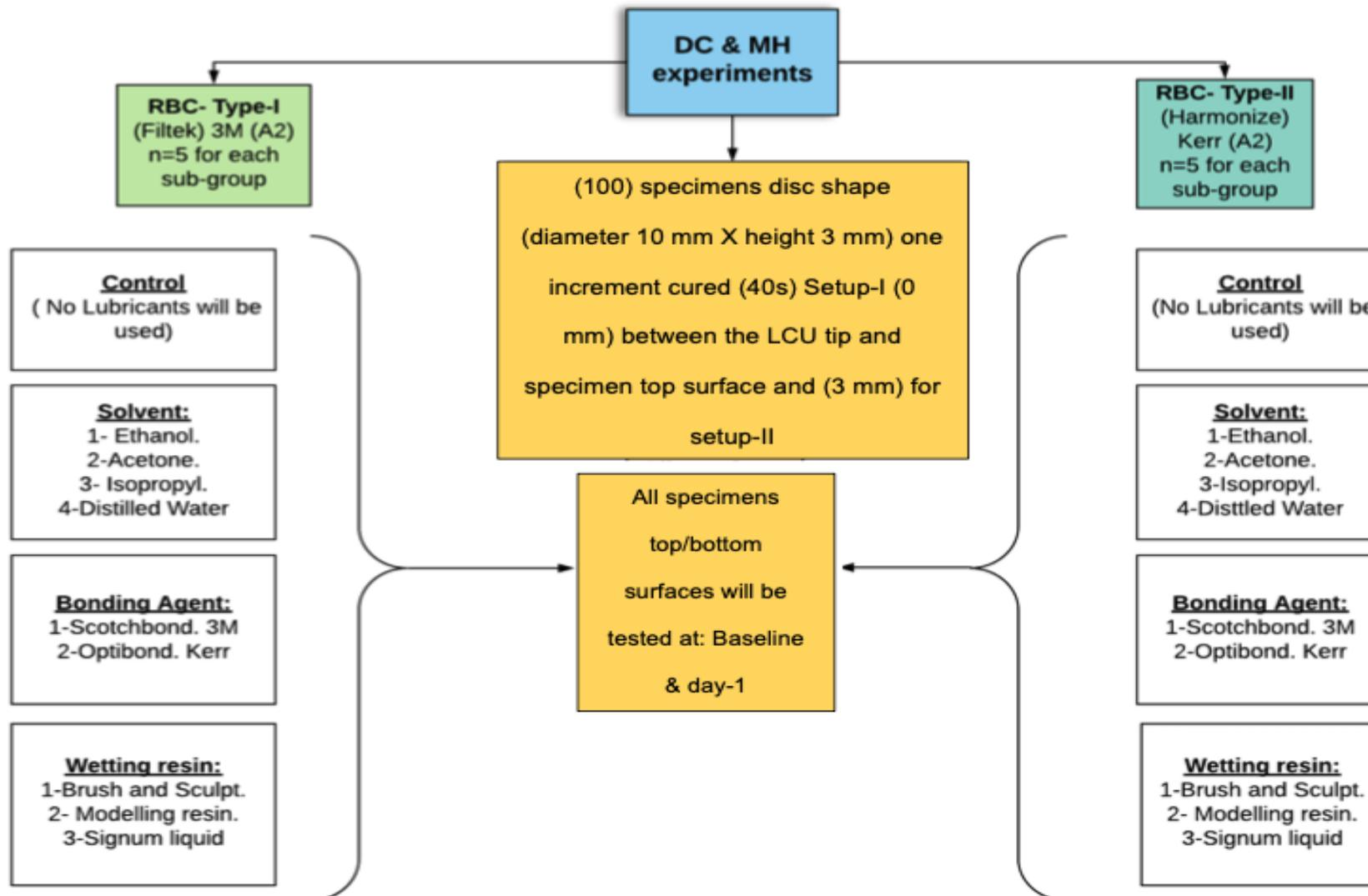
Figure 5-9: Specimen dimensions and key data for the degree of conversion and hardness experiments
