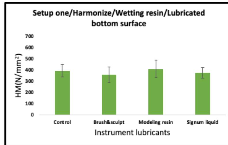
**Figure 5-40:** Mean and standard deviation values for tests of Martens hardness (Filtek & Harmonize) for non-lubricated top surface and wetting resin-lubricated bottom surface in setup one
