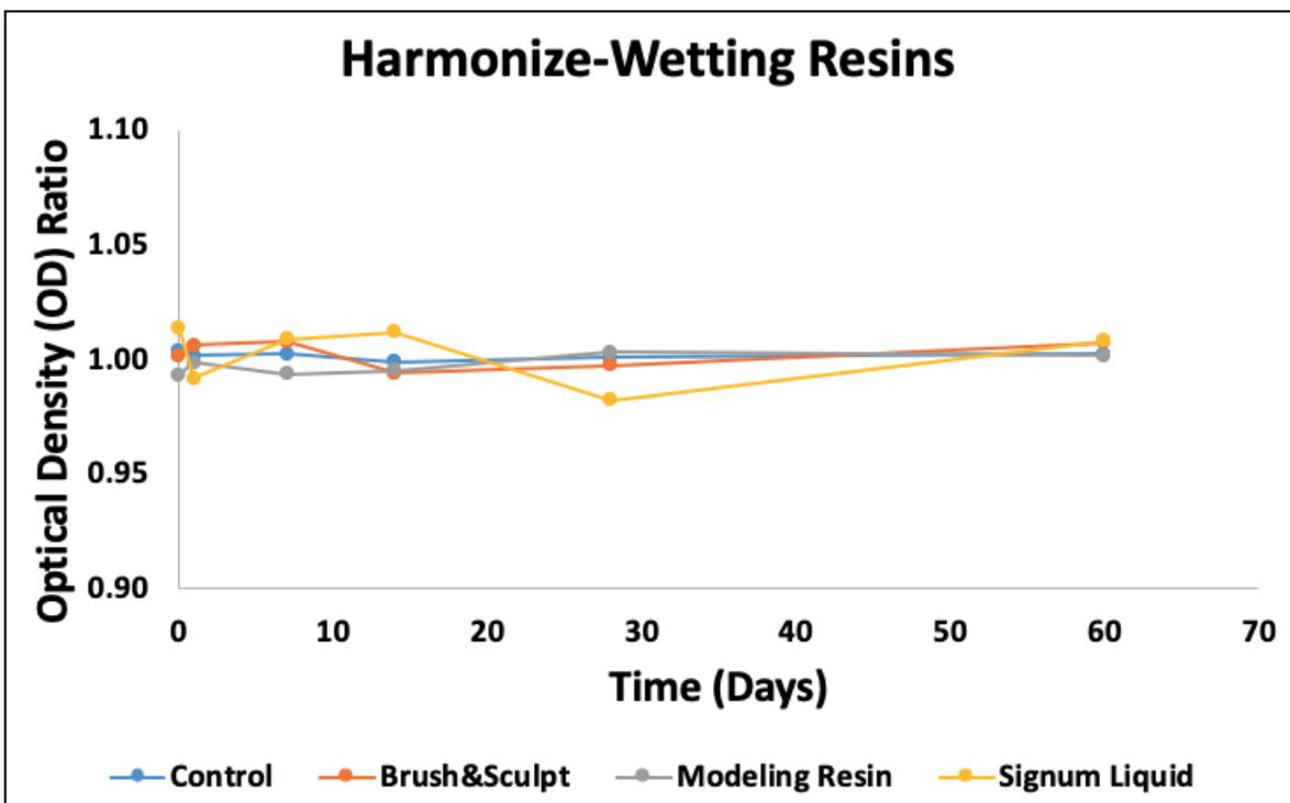
Figure 5-29: Optical density ratio of wetting resins over time for Filtek and Harmonize
