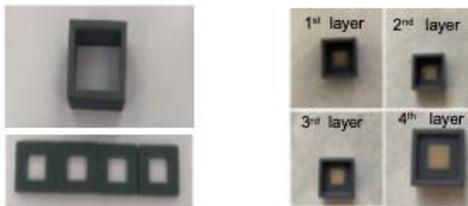
Figure-1: The mould layers and block building up. (each layer 2.5mm thickness)
