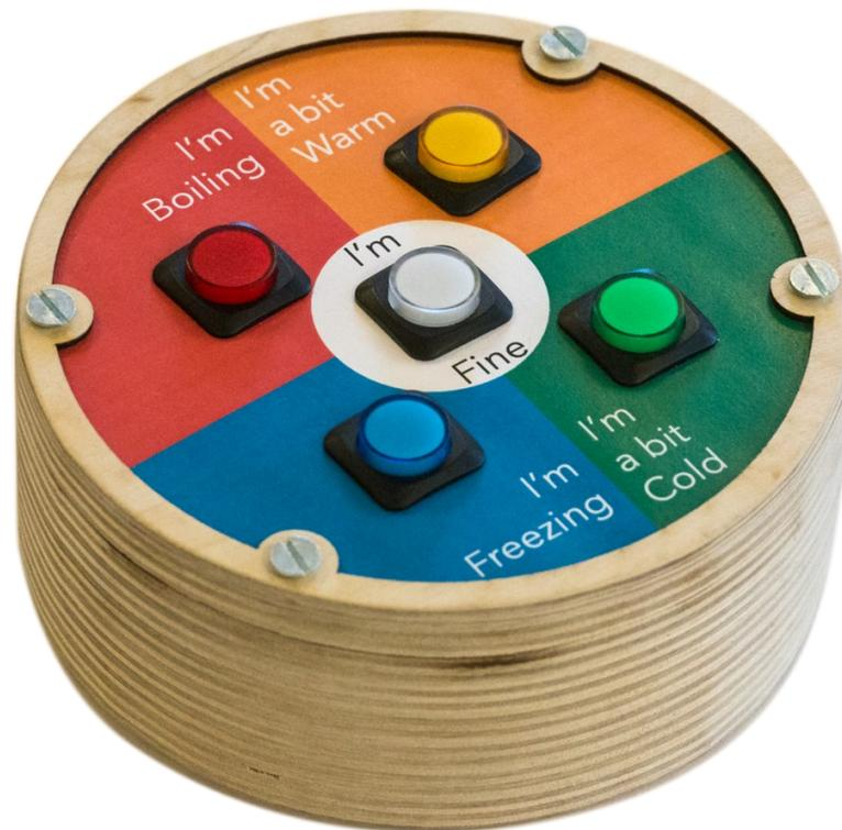
Figure 10: The ThermoKiosk survey device presenting users with a five-point Likert-type scale of thermal comfort by which to represent their experiences
