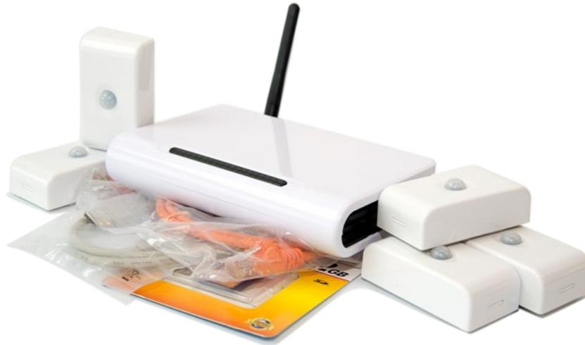
Figure 4: *BuildAX Environmental Sensor Toolkit: including logger, sensor nodes and supplied cables*
