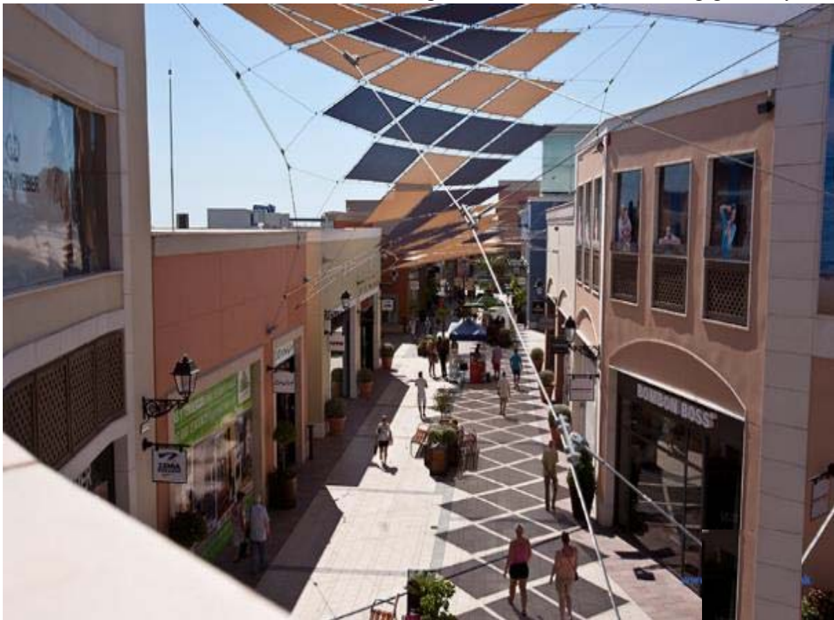
Figure 7.7: Horizontal shading device across the canyon's width providing shade to pedestrians
