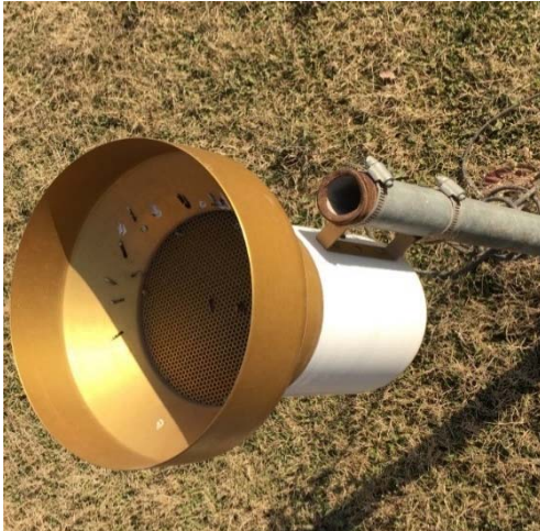
Figure8: .shows Rain gauge sensor TR-525M.(CampbellScientific 2017)
