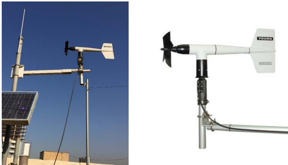
Figure7: .shows Wind speed and direction sensor 05106.(CampbellScientific 2017)
