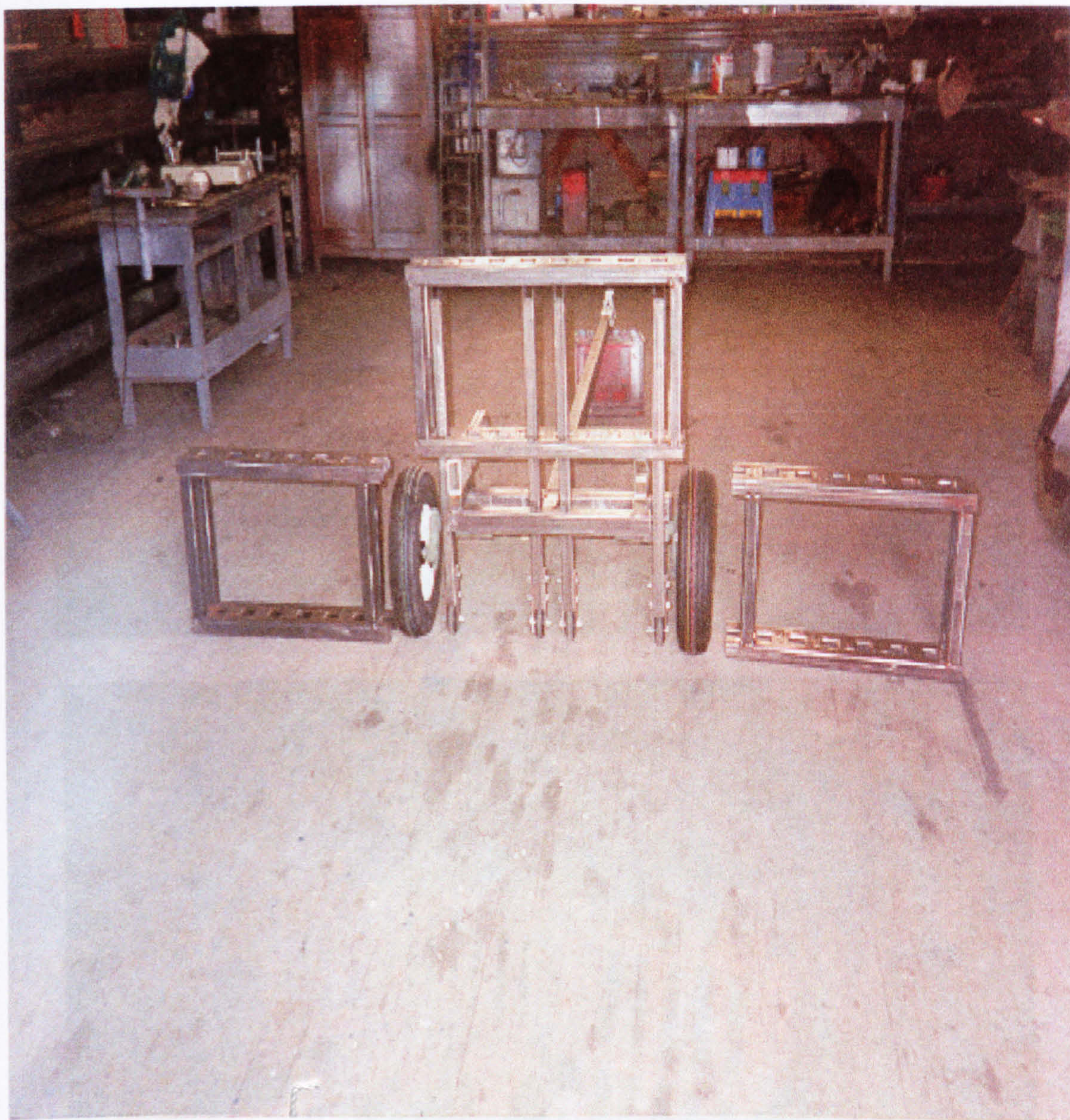
Figure 5.17 Splitting the main body to three parts
