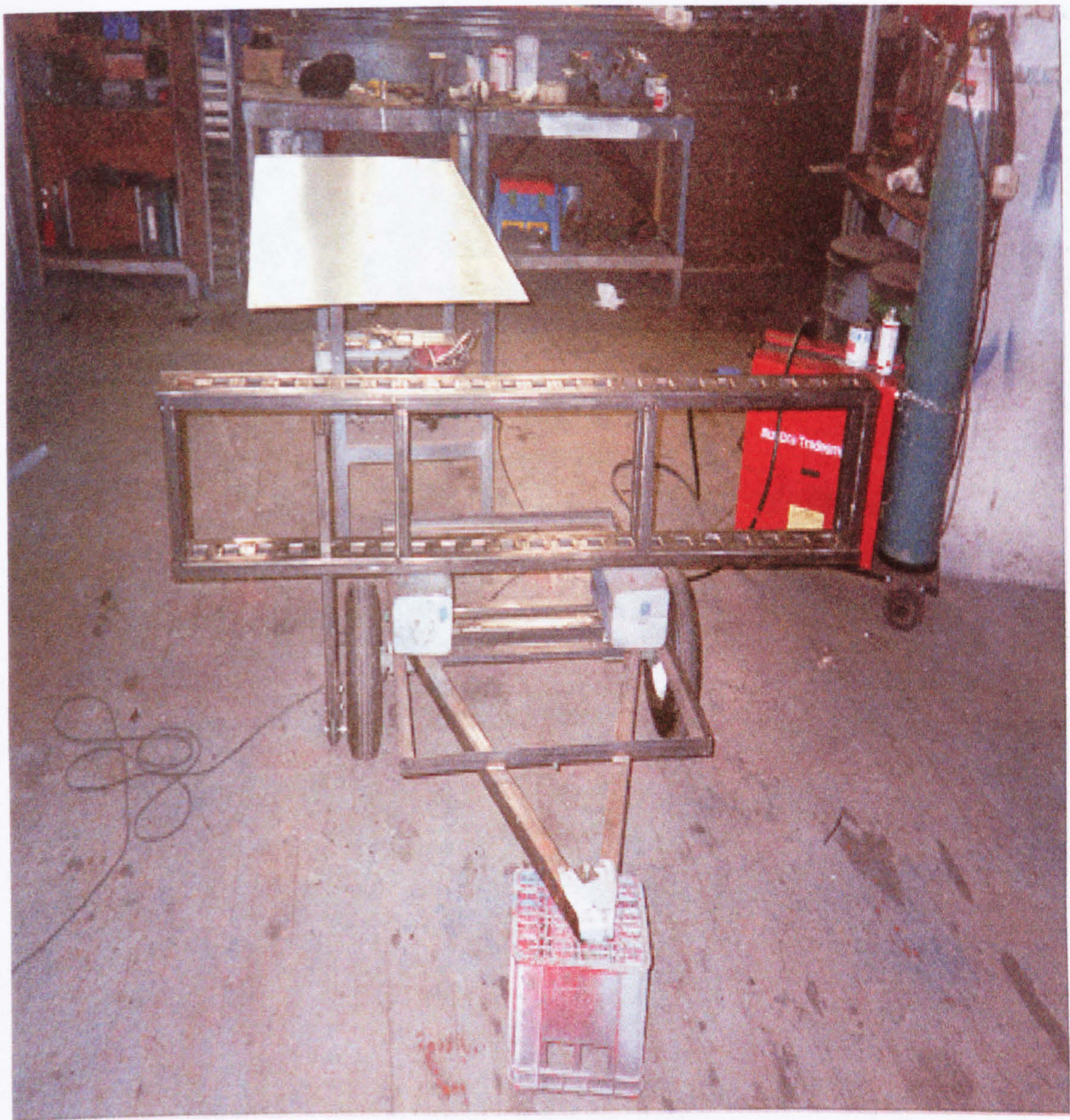
Figure 5.16 Positioning the main body on line with the trailer axle
