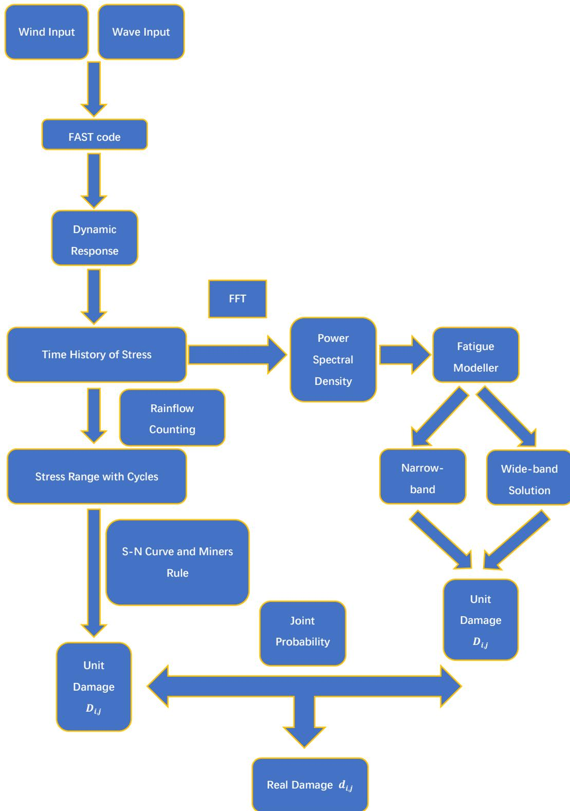
Figure 3.1 S-N curves based fatigue assessment procedure
