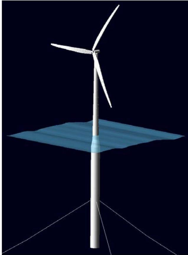
Figure 3.4 Configuration of spar-type FWT (Jonkman, 2010)
