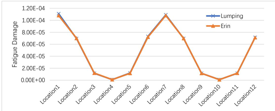
Figure 3.8 1-hour fatigue damage calculated by Erin et al., (2014) and joint lumping approach under 18 m/s of wind speed, 5 m of significant wave height and 14 s of peak period
