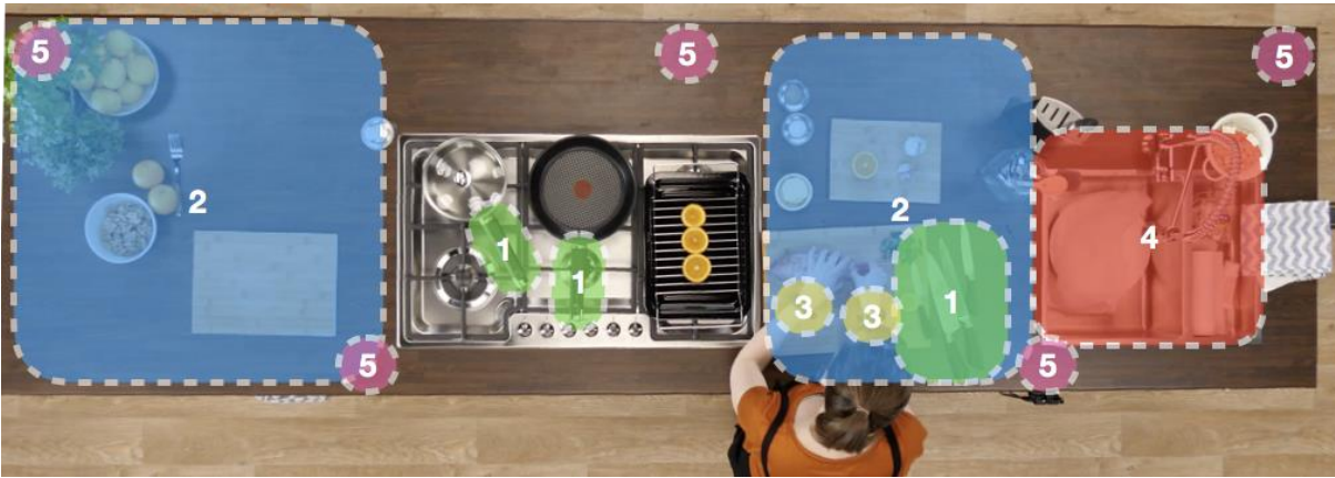
Figure 8. MoT Kitchen Sensing: (1) Accelerometers in utensils, pots and pans; 2. RFID positional information on ingredients and cookware; (3) IMU on chef's wrists; (4) Water flow meter on sink tap; (5) Bluetooth beacons for position of chef.
