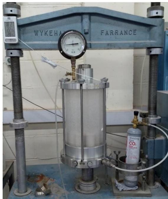
*Figure 3.3 Cylindrical specimens undergoing carbonation*
