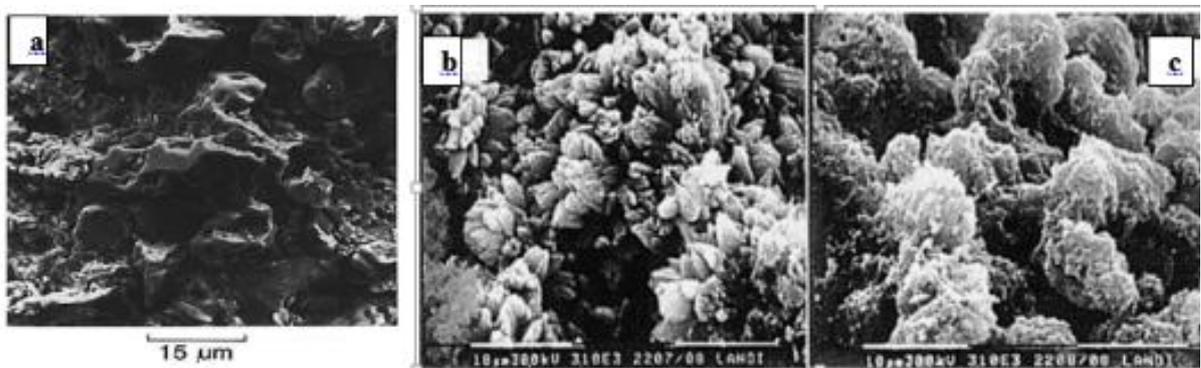
Figure 2.18 Carbonate connectors under scanning electron microscope **a**, authigenic calcite in Melan loess, China (adopted from Derbyshire and Mellors (1988)) **b**&**c**, pedogenic carbonates in Saskatchewan soils, Canada (adopted from Landi et al. (2003)).
