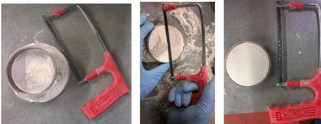
Figure A4-1 Calcareous oedometric specimen shaved into ring from a bulk-carbonated high-density sample
