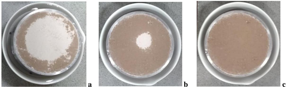
Figure 5.1 Solution absorption in oedometer specimens: a, b and c are different stages of the absorption process
