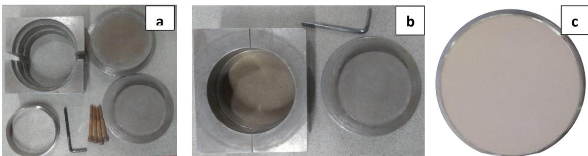
Figure A4-2 Split mould components for moulding low dry density oedometric specimens (a) components (b) assembled (c) specimen compacted into ring
