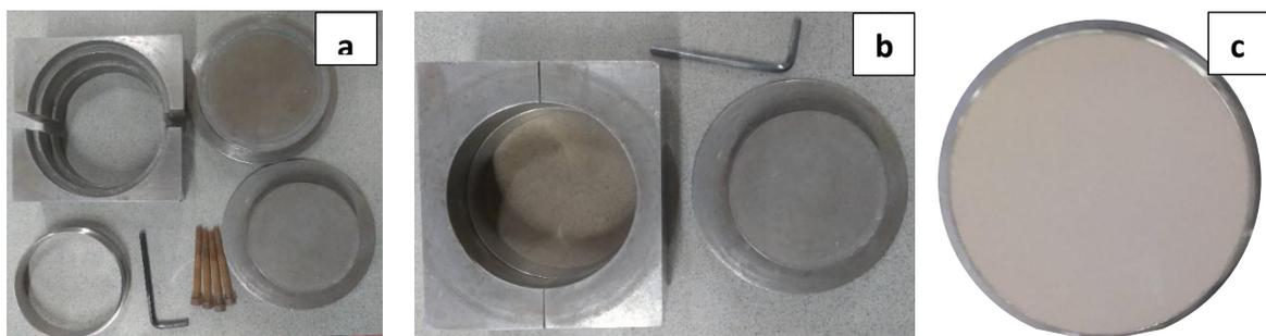
Figure A4-2 Split mould components for moulding low dry density oedometric specimens (a) components (b) assembled (c) specimen compacted into ring
