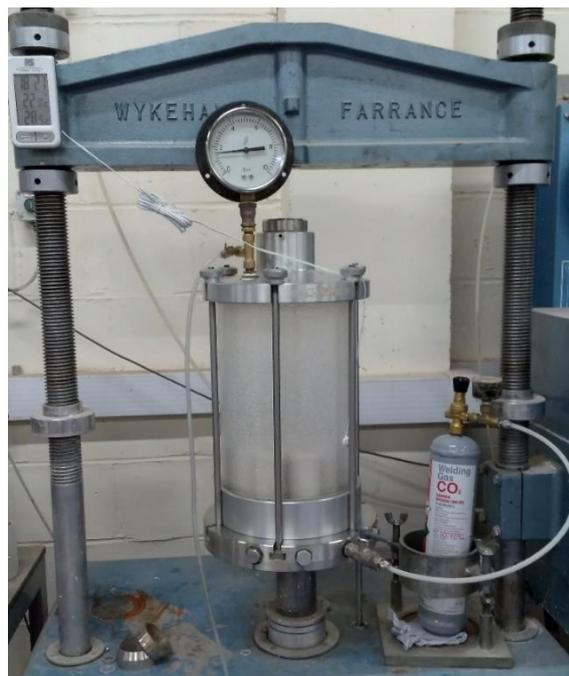
*Figure 3.3 Cylindrical specimens undergoing carbonation*
