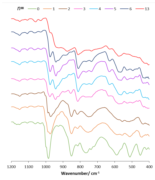
Figure 2.44 FTIR spectra of the solids isolated from the reactions between \text{V}_{13} and n mole-equivalents of Li|Hg amalgam in MeCN.
