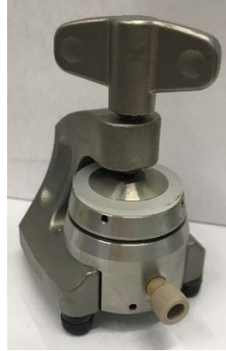
Figure 4.16 Schematic showing the two-electrode set up for an asymmetric supercapacitor.
