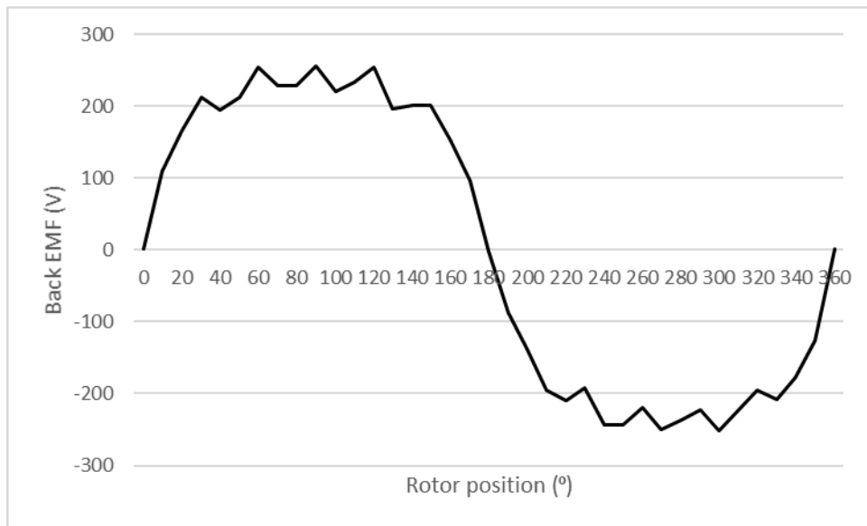
Figure 4. 18 Back EMF for open slot CW IPM Motor
