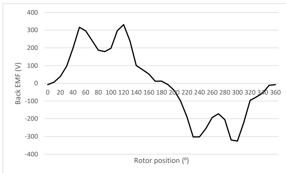
Figure 4. 19 Back EMF for semi-closed slot CW IPM motor
