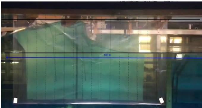
Figure 15 Calculation of the rise-up of a breaking wave via a tracker
