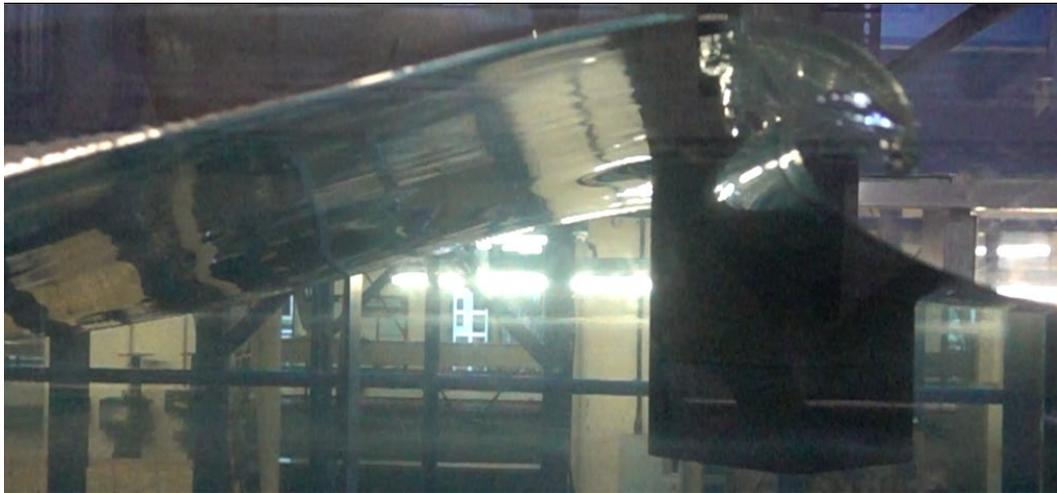
Figure 49 Plunging wave impact on diamond cylinder
