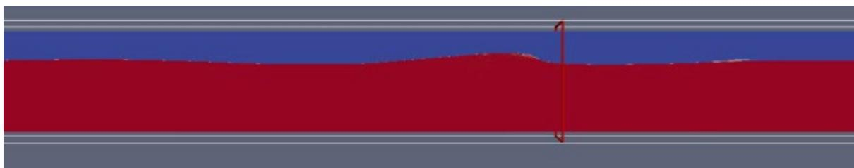
Figure 91 Early indication of formation of jet (using alpha\_water representation), a red rectangle box is placed at  $x = 9m$  for visualization purpose
