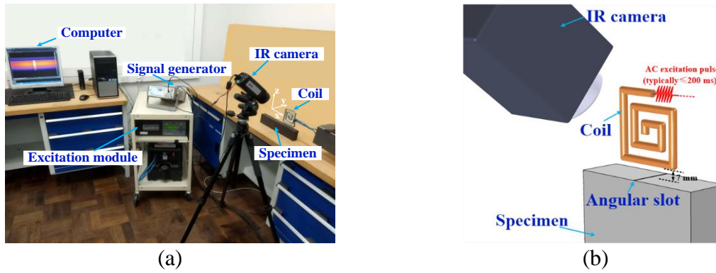
Figure 4.3 ECPT configuration for angular defect characterisation. (a) Layout of ECPT configuration. (b) Schematic diagram of ECPT configuration.
