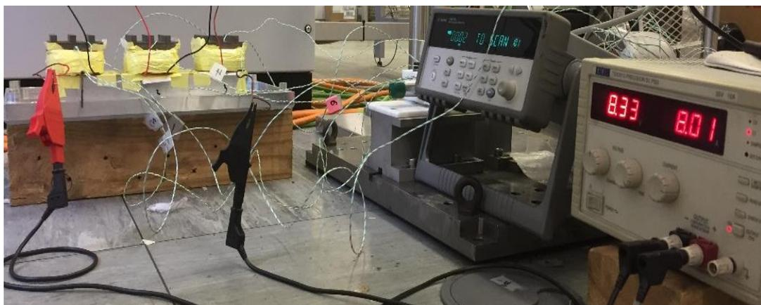
Figure 4. 55: Thermal testing of three-phase winding.
