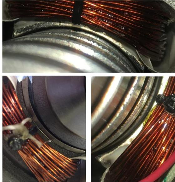
Figure 5.27: The three air-gap regions of the prototype under three stator teeth.
