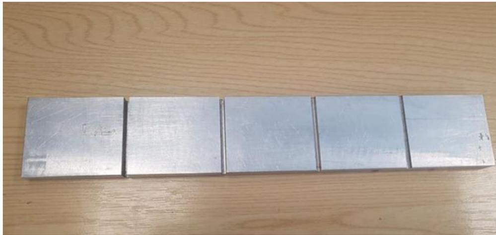
Figure 6.3 Aluminium test sample with artificial cracks
