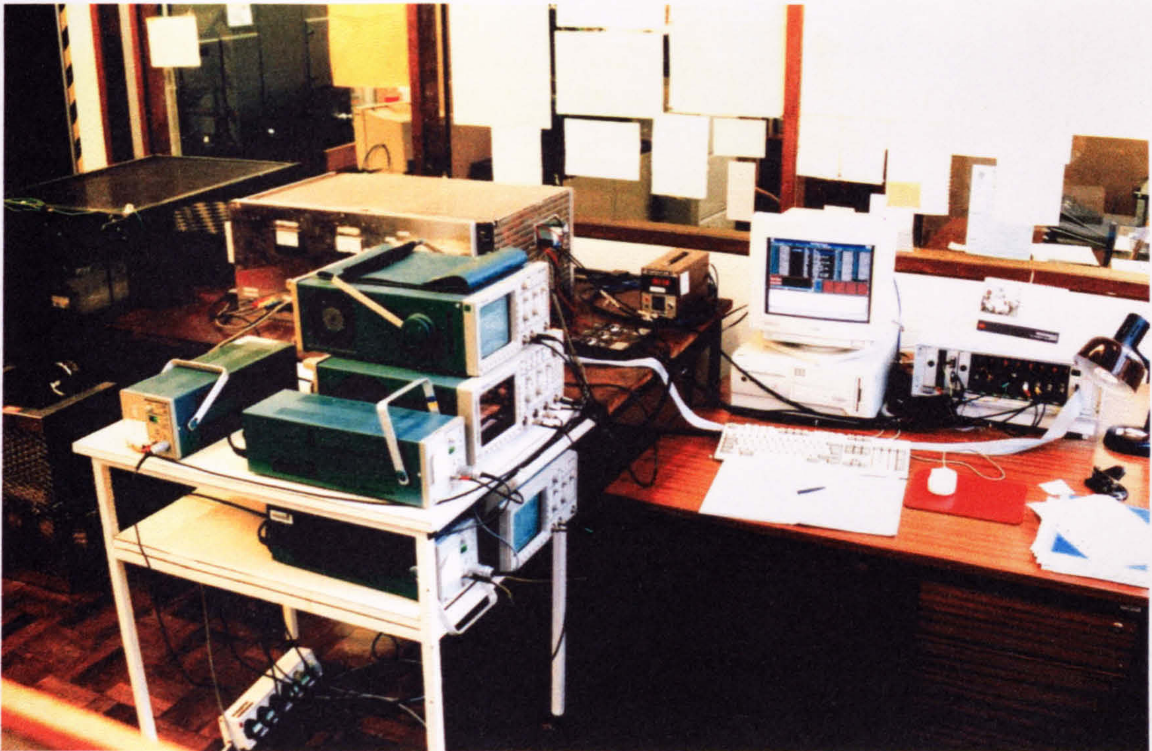
Figure E.1: The picture shows the complete test arrangement and converter. Left: Resistor bank and load inductors, Middle background: Converter, Centre front: Measurement equipment, Right: PC and controller unit.
