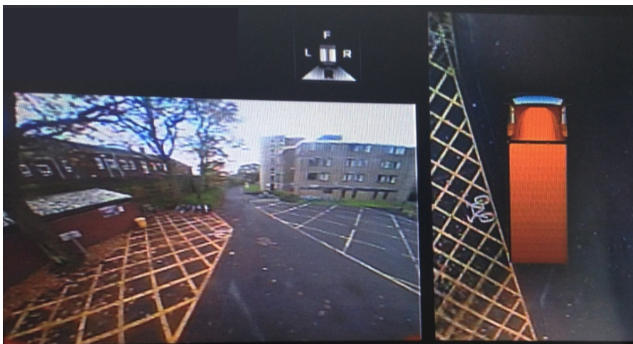
Figure 80: Brigade 360° - Camera view fitted to the vehicle. Source: Brigade Electronics system
