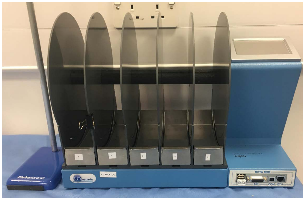
Figure 2.7. Rotarod device to measure latency to fall. The multi-lane device allowed for grip strength and coordination testing independently over three trials.
