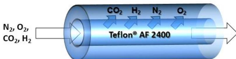
Figure 2.1 Teflon<sup>®</sup> AF-2400 based ‘tube-in-tube’ gas-liquid reactor.
