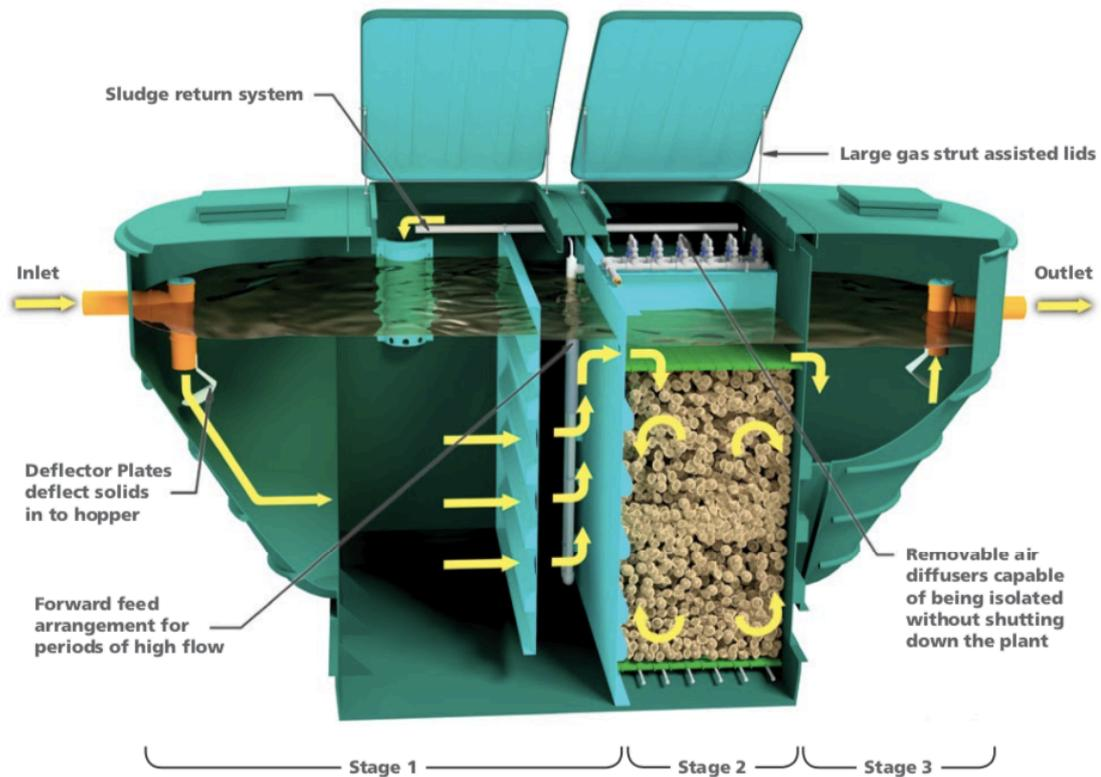
Figure 3 - Schematic of the WPL High Performance Aerated Filter (HiPAF) system WPL, (2019).
