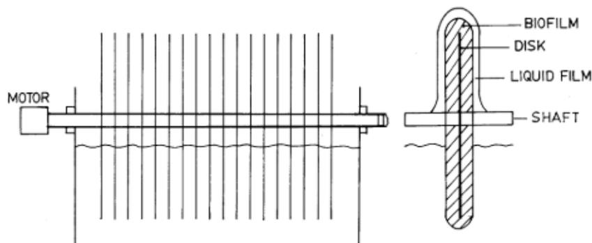
Figure 2 - Schematic of a single rotating biological contactor unit (Patwardhan, 2003).
