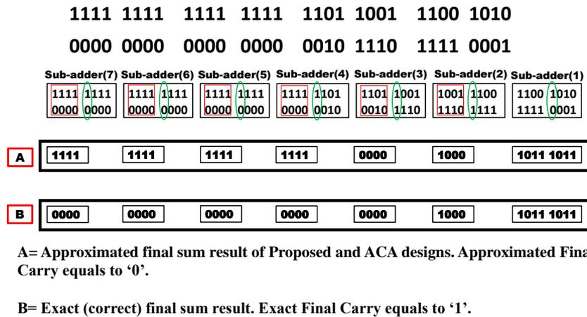
Figure 3.4: Proposed design numerical (32-bit) approximate addition example.
