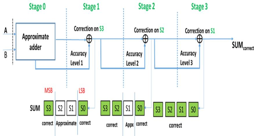
Figure 4.5: Significance-driven structure of error correction stages.
