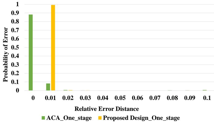
Figure 5.12: 32-Bit proposed design vs. ACA relative error distance (RED) distribution analysis (One correction stage).
