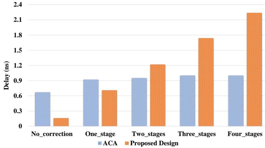
Figure 5.8: 32-Bit proposed design versions vs. ACA delay (ns) comparison.
