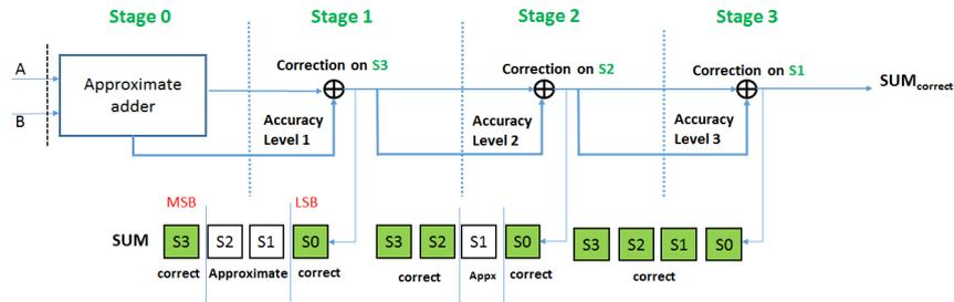
Figure 3.3: Significance-driven error correction stages (32-bit adder example).
