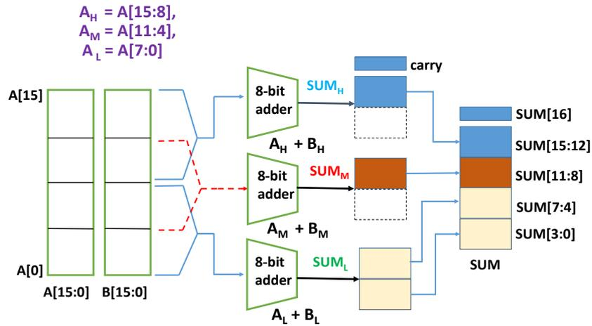
Figure 2.10: ACA adder example (16-bit adder), where H=High, M=Middle and L=Low.
