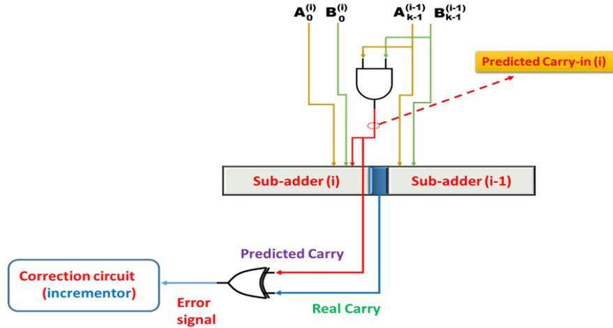
Figure 4.4: The proposed error detection technique augmented with the carry-in prediction circuit.
