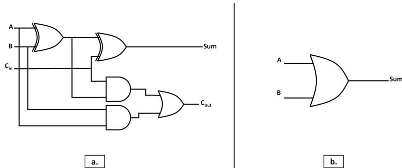
Figure 5.1: The conventional full adder circuit in (a.) versus the proposed approximate OR gates addition operation in (b.).
