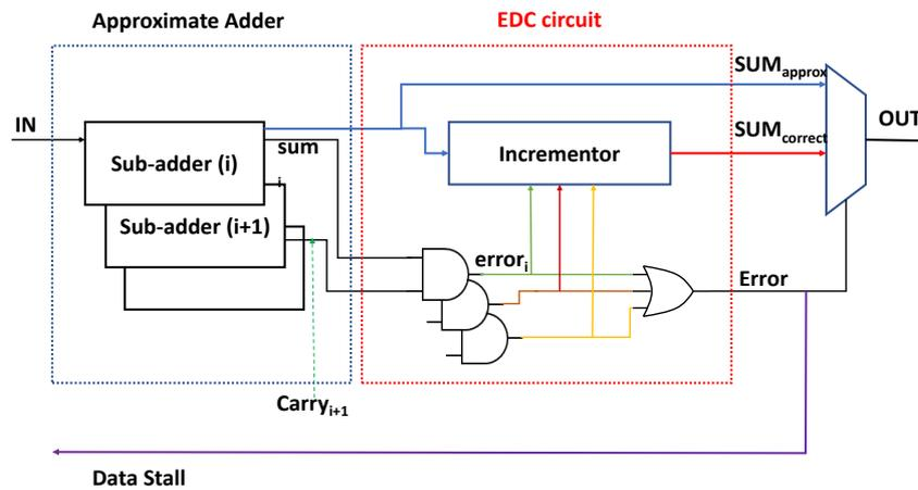
Figure 2.11: ACA error detection and correction circuit.
