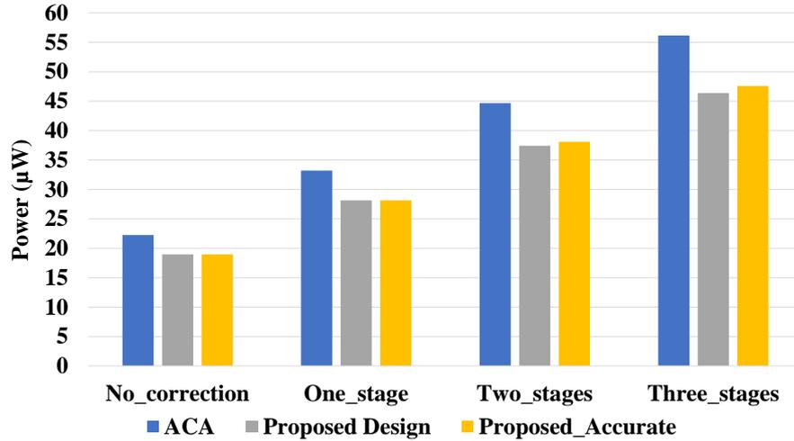
Figure 4.7: 32-Bit proposed design versions vs. ACA dynamic power ( $\mu\text{W}$ ) comparison.
