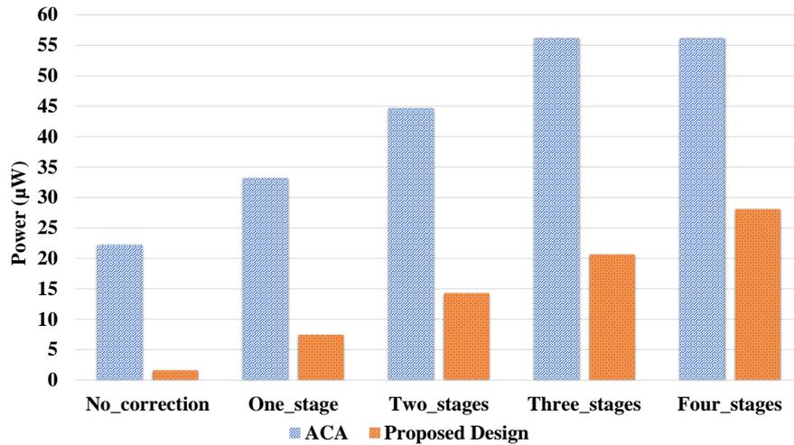
Figure 5.5: 32-Bit proposed design versions vs. ACA dynamic power ( $\mu\text{W}$ ) comparison.
