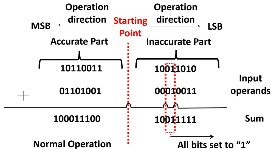
Figure 2.7: Error-tolerant adder (ETA).
