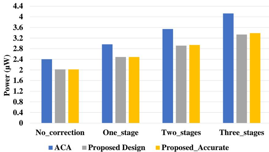
Figure 4.8: 32-Bit proposed design versions vs. ACA leakage power ( $\mu\text{W}$ ) comparison.
