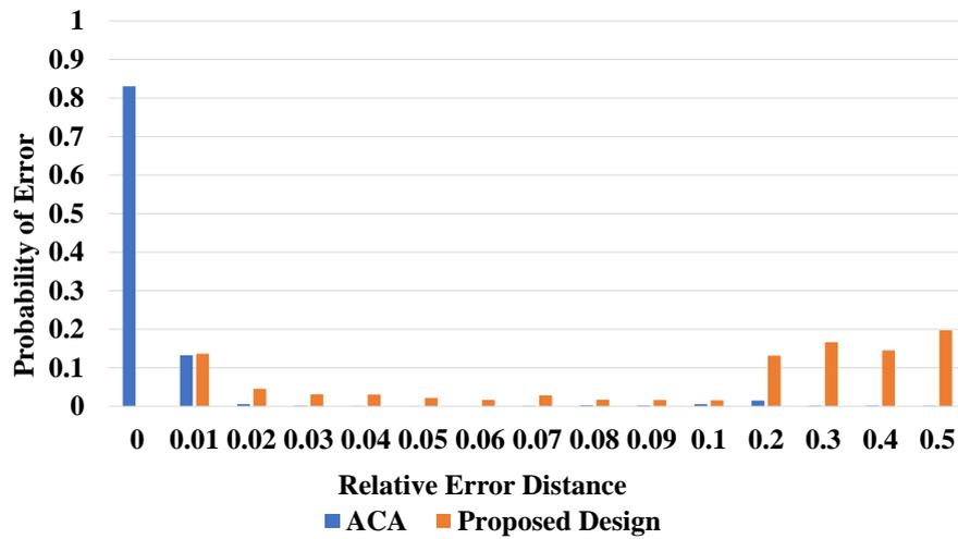
Figure 5.11: 32-Bit proposed design vs. ACA relative error distance (RED) distribution analysis (No correction stages).
