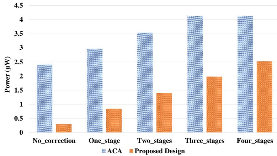
Figure 5.6: 32-Bit proposed design versions vs. ACA leakage power ( $\mu\text{W}$ ) comparison.
