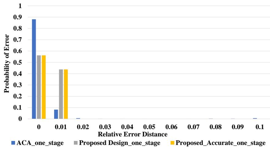
Figure 4.12: 32-Bit proposed design vs. ACA relative error distance (RED) distribution analysis (One correction stage).
