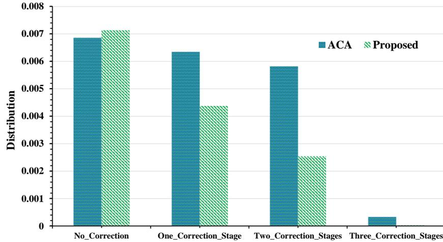
Figure 4.15: The 32-Bit adder designs MRED values comparison through different correction stages.
