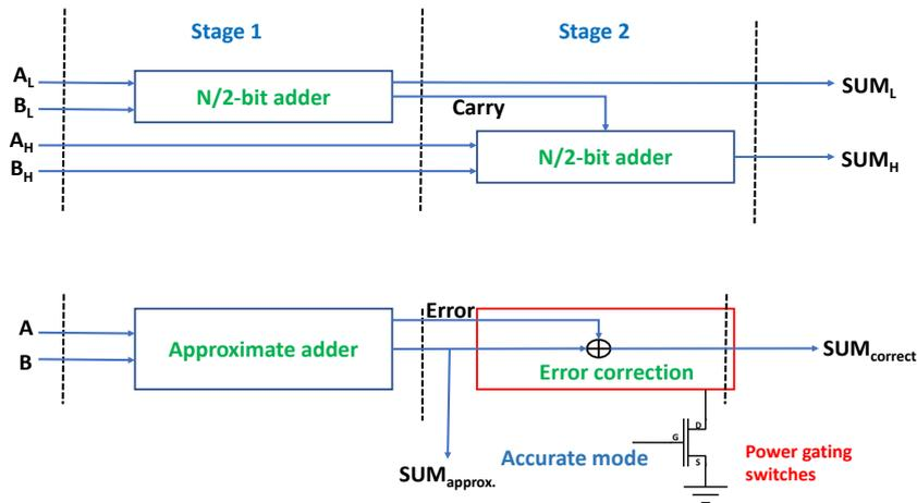
Figure 2.12: Two stages implementation of the approximate adder (below) with power gated correction stage, a conventional adder (above).
