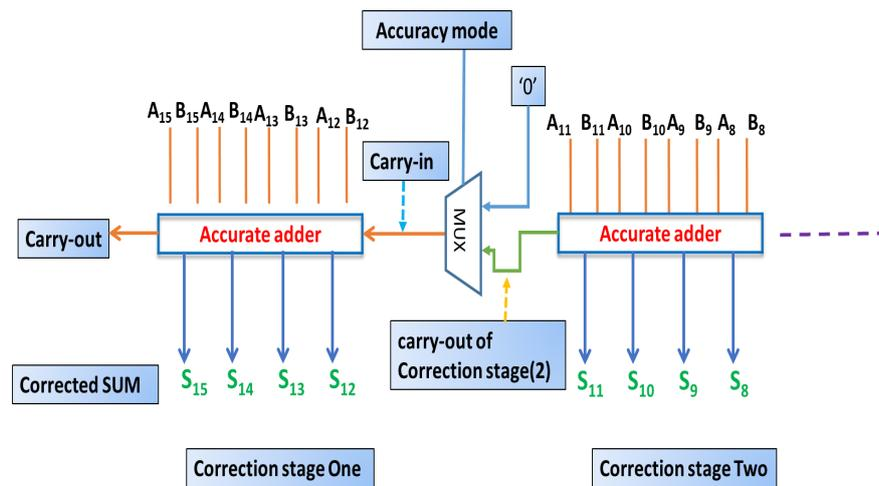
Figure 5.2: The proposed accuracy recovery circuit.
