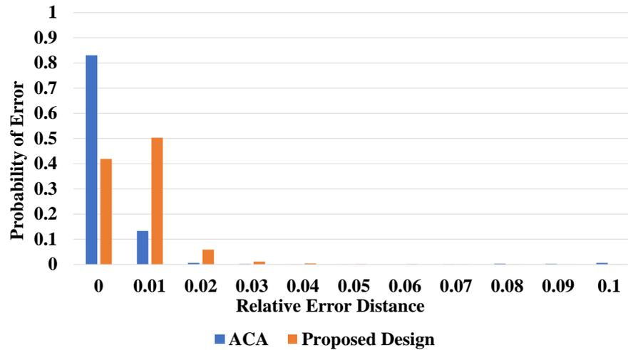
Figure 4.11: 32-Bit proposed design vs. ACA relative error distance (RED) distribution analysis (No correction stages).
