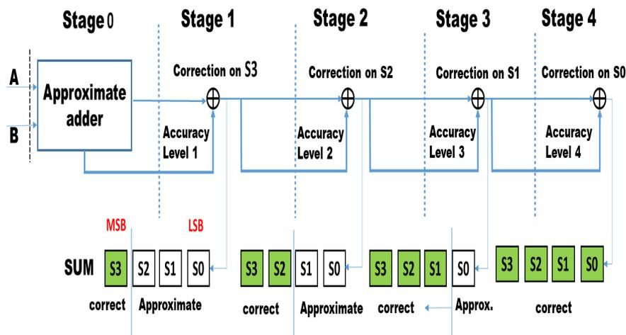
Figure 5.3: Significance-driven error correction stages (32-bit adder example).
