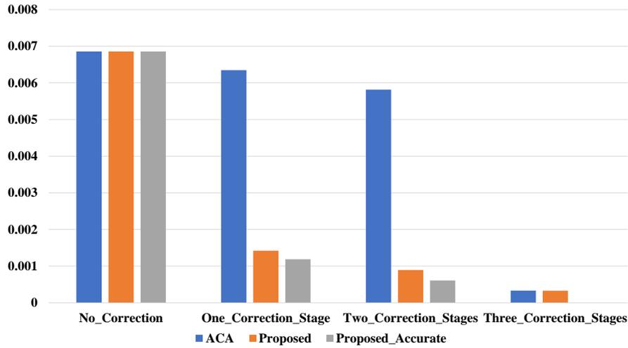
Figure 3.15: The 32-Bit adder designs MRED values comparison through different correction stages.
