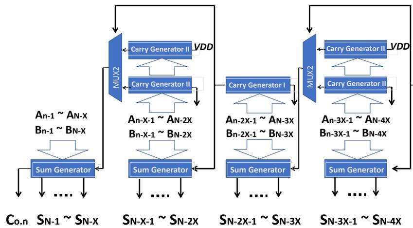
Figure 2.8: Block diagram of ETA type IV (ETAIV).
