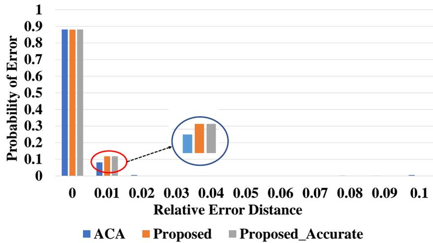
Figure 3.12: 32-Bit proposed design vs. ACA relative error distance (RED) distribution analysis (One correction stage).
