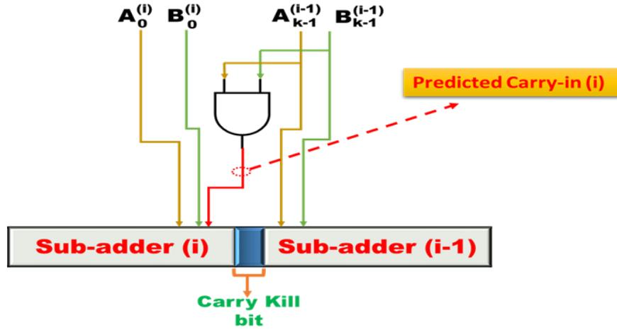
Figure 4.2: The proposed carry-in prediction technique for each segmented sub-adder.
