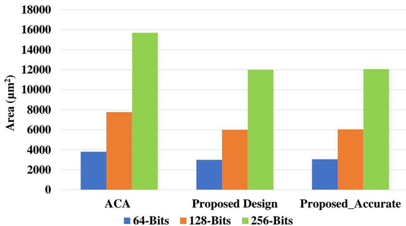
Figure 4.19: ACA vs. proposed large adder designs area ( $\mu\text{m}^2$ ) comparison.
