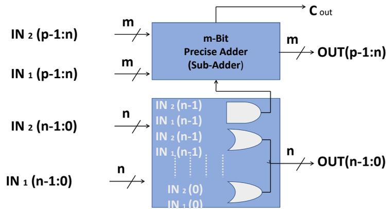
Figure 2.6: Lower-Part-OR adder (LOA) architecture.
