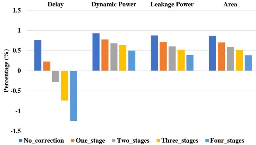
Figure 5.9: 32-Bit proposed design vs. ACA reduction ratio values.
