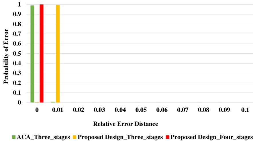
Figure 5.14: 32-Bit proposed design vs. ACA relative error distance (RED) distribution analysis with three and four correction stages.
