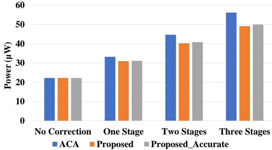
Figure 3.6: 32-Bit proposed design versions vs. ACA dynamic power ( $\mu\text{W}$ ) comparison.
