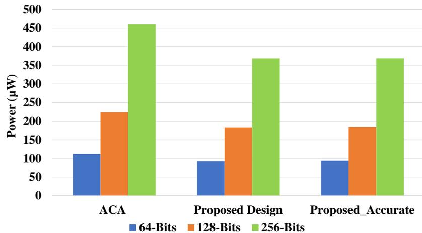
Figure 4.17: ACA vs. proposed large adder designs dynamic power( $\mu$ W) comparison.
