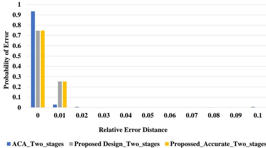
Figure 4.13: 32-Bit proposed design vs. ACA relative error distance (RED) distribution analysis (Two correction stage).
