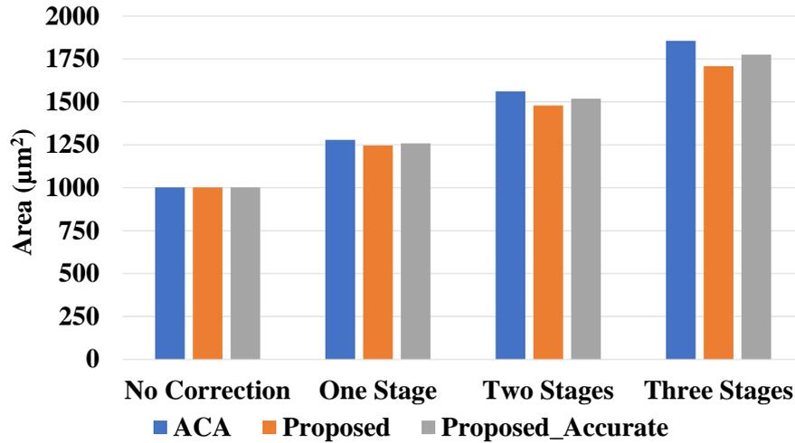
Figure 3.8: 32-Bit proposed design versions vs. ACA area ( $\mu\text{m}^2$ ) comparison.
