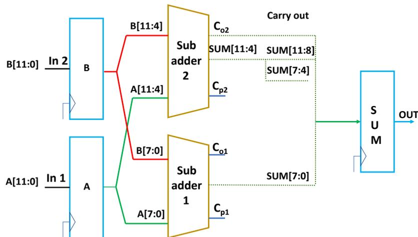
Figure 2.13: GeAr adder with  $N=12$ ,  $R=4$ ,  $P=4$  and  $M=2$ .
