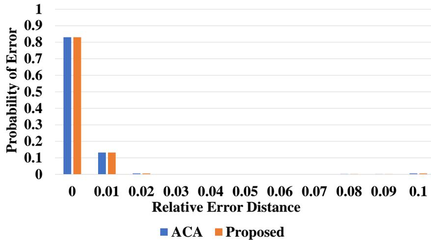
Figure 3.11: 32-Bit proposed design vs. ACA relative error distance (RED) distribution analysis (No correction stages).
