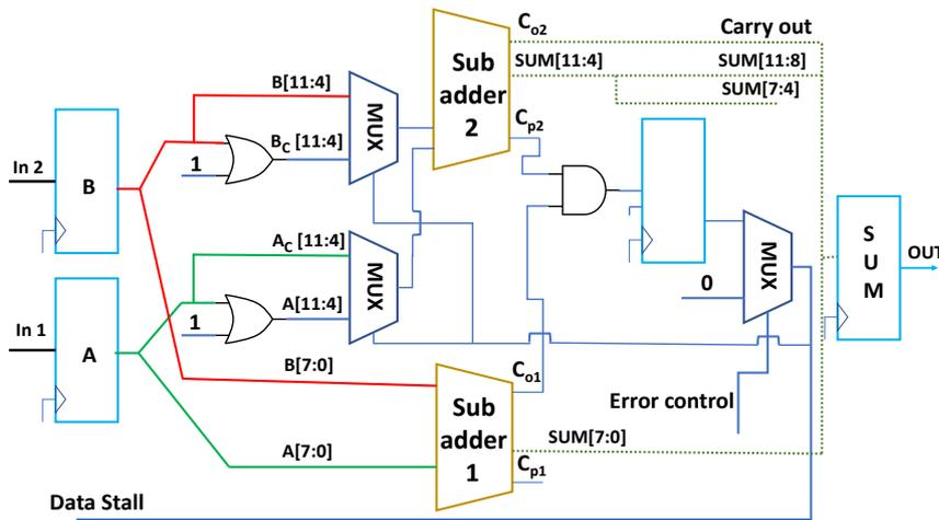
Figure 2.15: Error detection and correction for GeAr adder with  $N=12$ ,  $R=4$ ,  $P=4$  and  $k=2$ .
