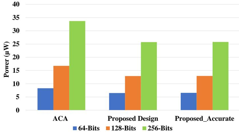
Figure 4.18: ACA vs. proposed large adder designs leakage power ( $\mu\text{W}$ ) comparison.
