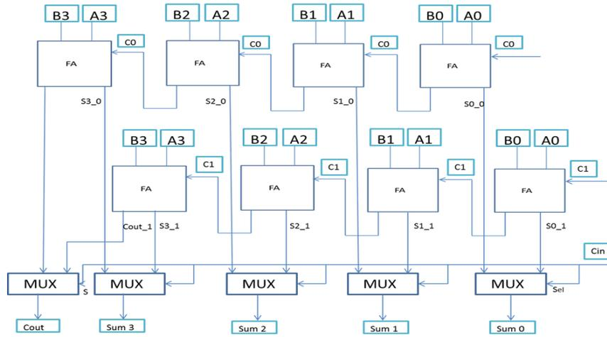
Figure 2.3: 4-Bits carry select adder.
