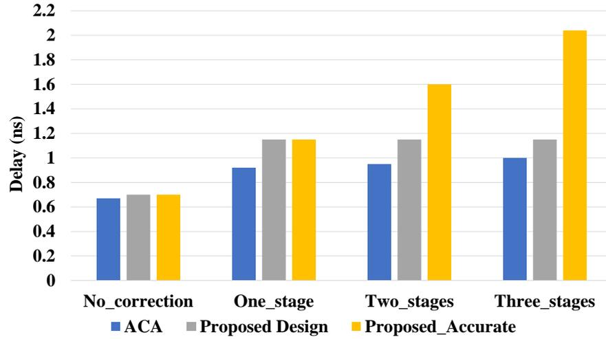
Figure 4.10: 32-Bit proposed design versions vs. ACA delay (ns) comparison.
