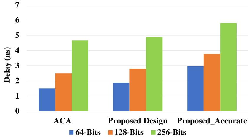
Figure 4.20: ACA vs. proposed large adder designs delay (ns) comparison.
