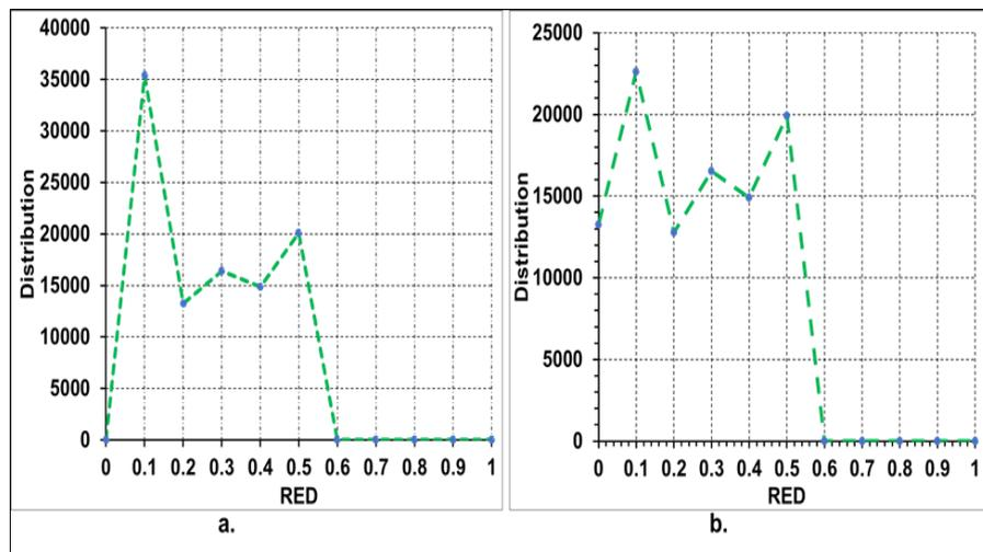
Figure 5.10: Monte Carlo analysis of logic OR addition implementation in (a) 32-bit inputs, and (b) 8-bit inputs.
