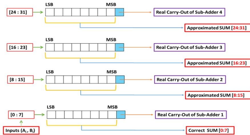
Figure 4.3: Example of (32-bit) proposed approximate adder using the segmenting technique of carry kill bit locations.
