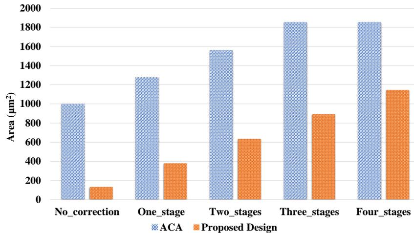
Figure 5.7: 32-Bit proposed design versions vs. ACA area ( $\mu\text{m}^2$ ) comparison.
