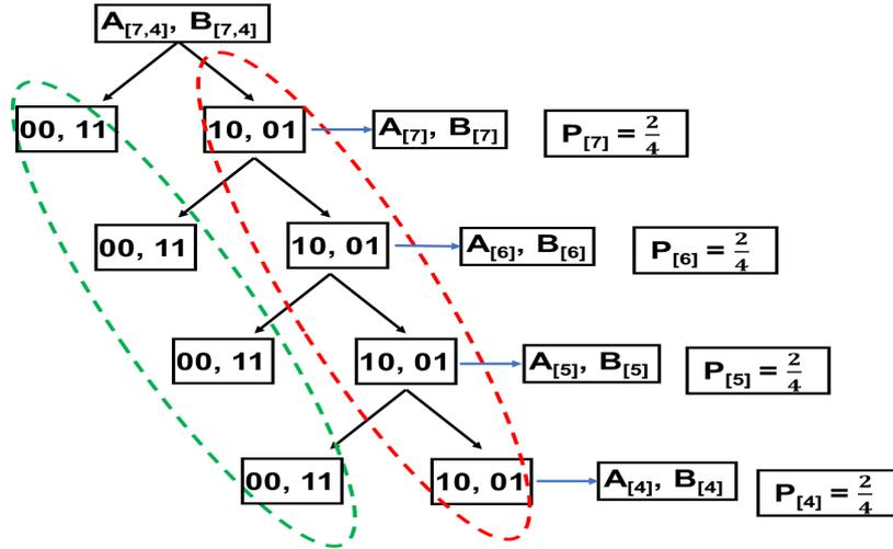
Figure 3.10: Tree of probability of carry propagation based on inputs bits values assuming C1= '1' and C2= '0'.
