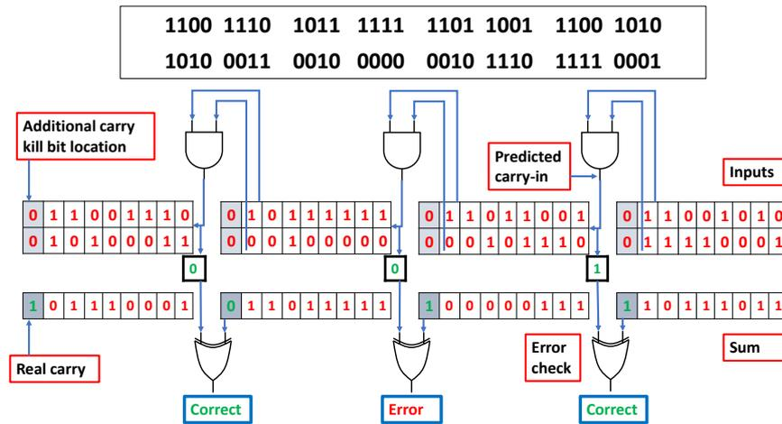
Figure 4.6: Proposed design numerical example of (32-bit) inputs addition, sub-adders carry-in prediction and error (carry propagation) detection.
