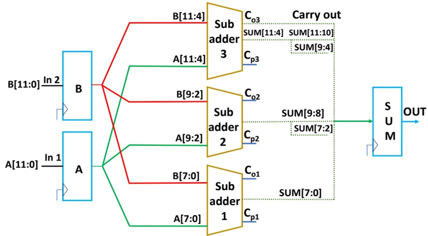
Figure 2.14: GeAr adder with  $N=12$ ,  $R=2$ ,  $P=6$  and  $M=3$ .
