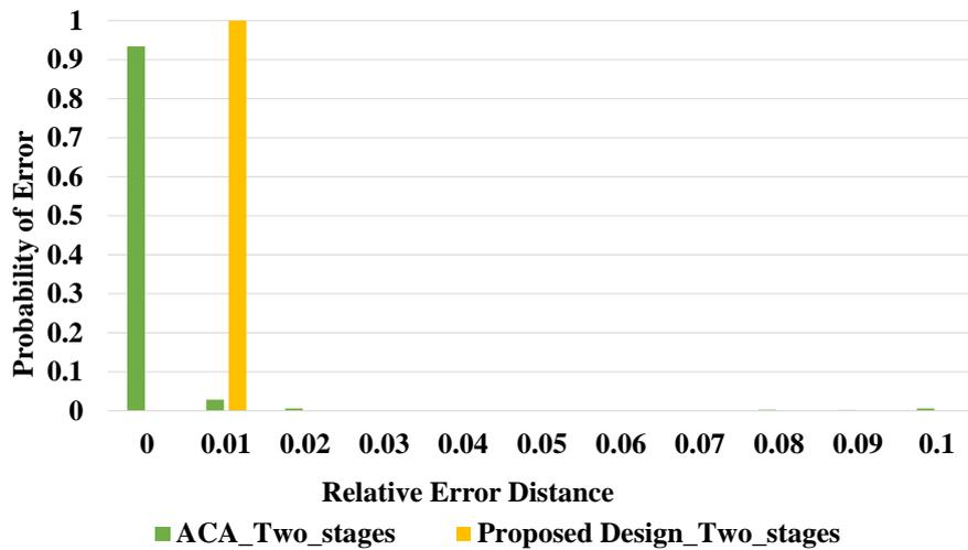
Figure 5.13: 32-Bit proposed design vs. ACA relative error distance (RED) distribution analysis (Two correction stage).
