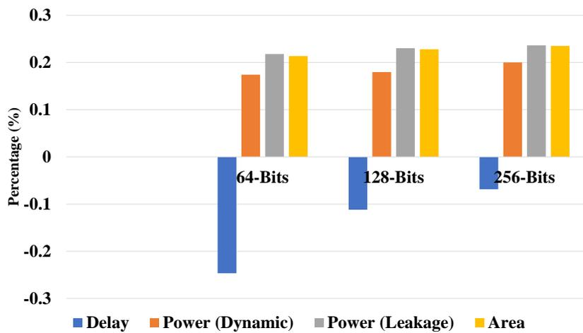
Figure 4.21: ACA vs. proposed large adder designs reduction ratio values.
