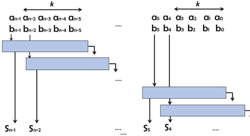
Figure 2.9: VLSA single-bit shift segmentation.
