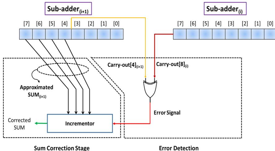
Figure 3.2: Proposed error detection technique.
