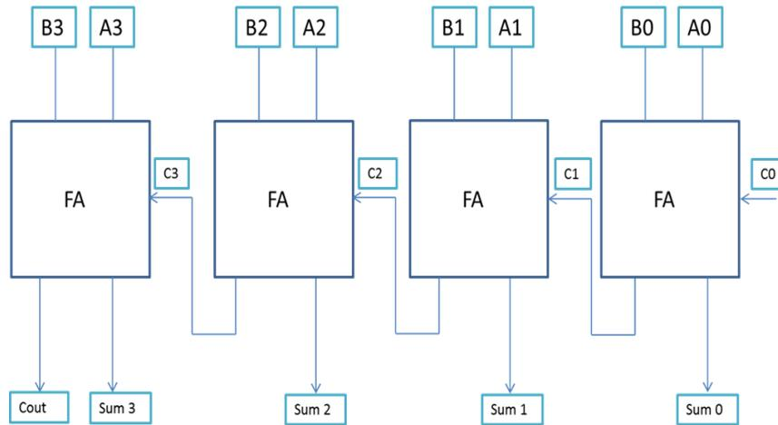
Figure 2.2: 4-Bits ripple carry adder.
