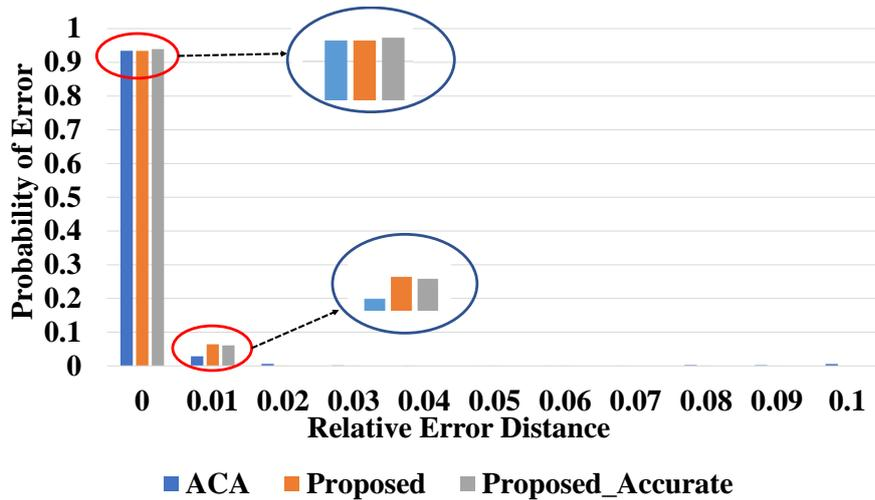
Figure 3.13: 32-Bit proposed design vs. ACA relative error distance (RED) distribution analysis (Two correction stages).
