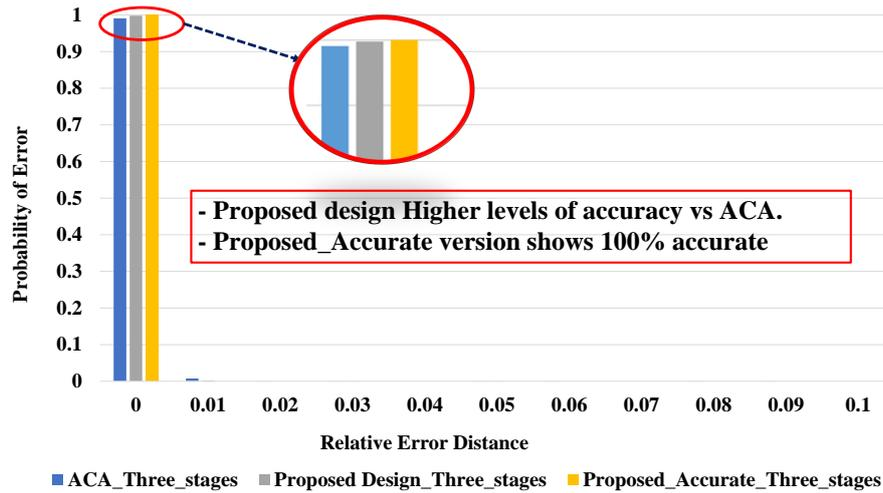
Figure 4.14: 32-Bit proposed design vs. ACA relative error distance (RED) distribution analysis (Three correction stage).
