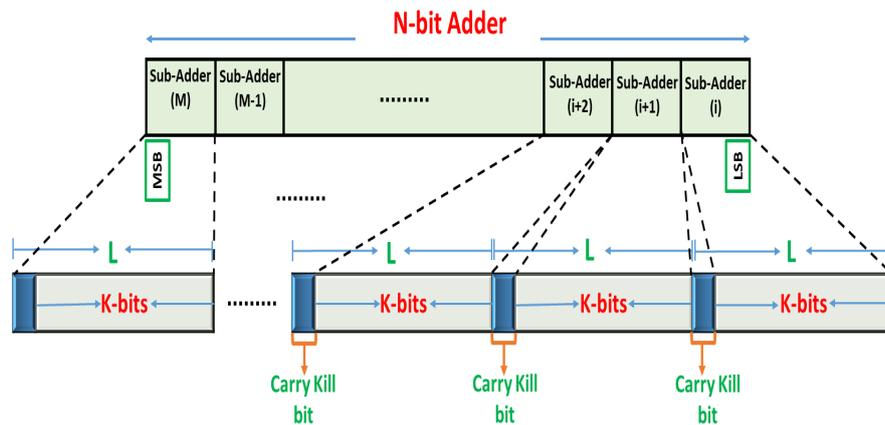
Figure 4.1: The proposed general adder segmentation technique using the carry kill new bit locations.
