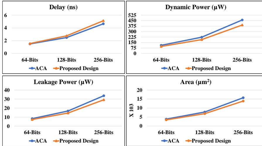
Figure 3.17: ACA vs. Proposed large bit-width adder designs hardware comparisons.
