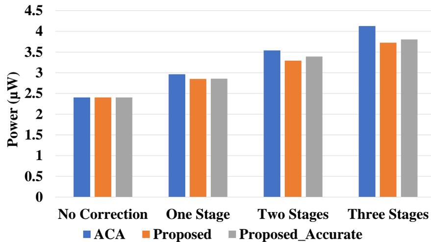
Figure 3.7: 32-Bit proposed design versions vs. ACA leakage power ( $\mu\text{W}$ ) comparison.
