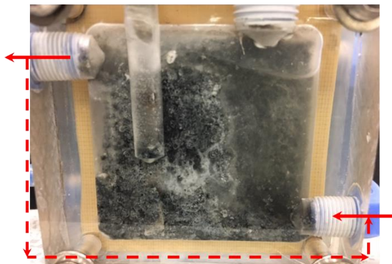
Figure 5.9 Biocathode after the experiments. White crystallisation and black biomass were appeared on the surface of the electrode causing current density dropped. Line arrows show inlet and outlet direction. Dash line arrows are recycling flows.
