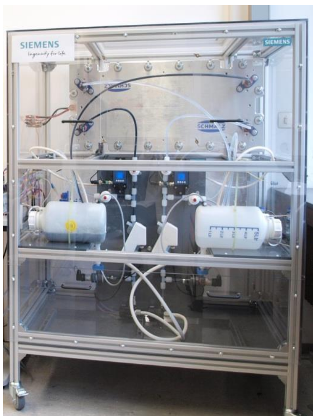
Figure 51 Photograph of the 1400 cm 2 cell with periphery (tanks, pumps, tubing) and containment.
