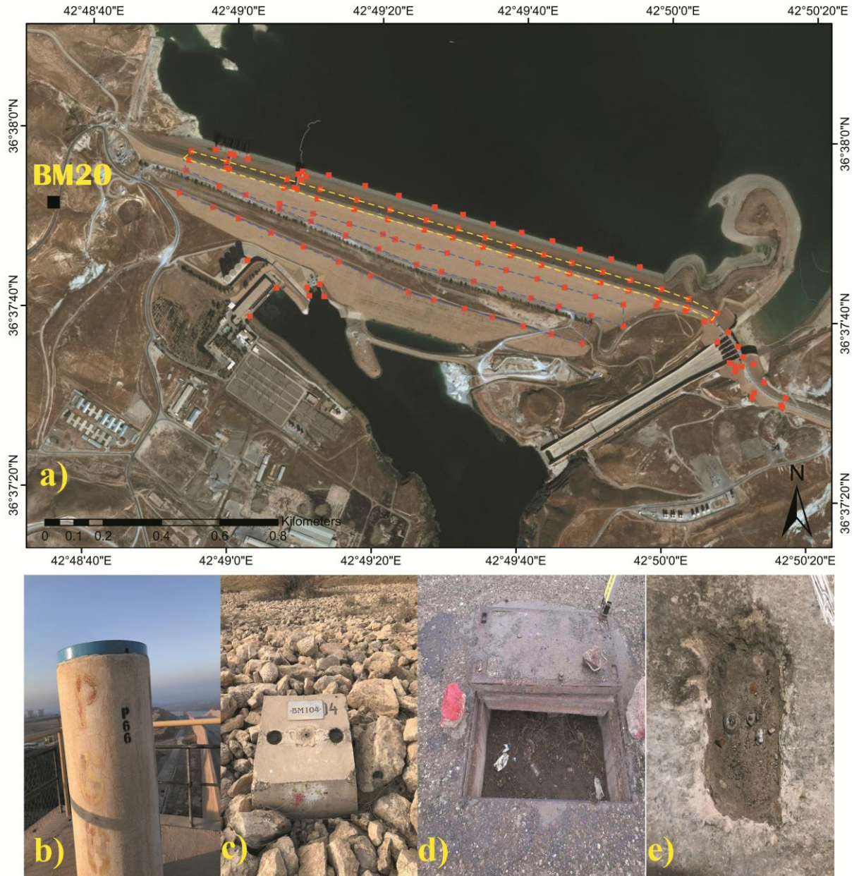
Figure 4.2. The vertical geodetic network of Mosul dam: a) location of BMs on the Mosul dam, where dashed lines refer to the levelling loops which are used in geodetic levelling monitoring. Background image from (Esri, DigitalGlobe 2018), b) monument pillar of the horizontal network, c) BM on the dam slope; d) BM on the dam crest; e) BM on the gallery.
