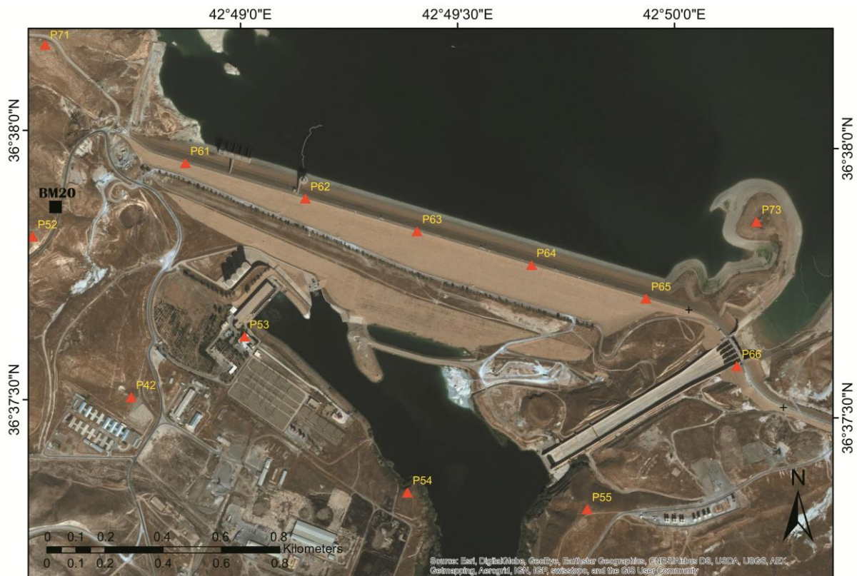
Figure 4.1. The horizontal geodetic network of the Mosul dam. The monitoring pillars P1-P6 are monitored using the other reference pillars on the dam site. Background image from (Esri, DigitalGlobe 2018).
