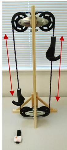
**Figure 2-2: A two-sided pulley for a closed-loop FES task**
