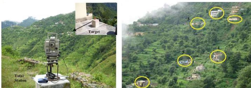
Figure 2-15: (a) A total station and (b) the establishment of targets for landslide movement monitoring in slope areas (Sarkar *et al.*, 2013).
