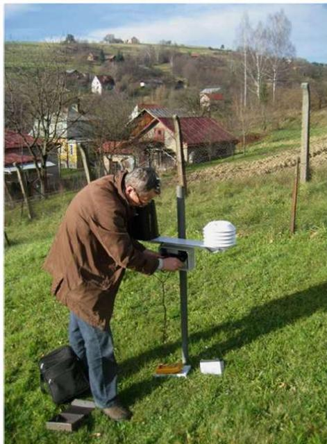
Figure 2-11: Example of a weather station, including rainfall gauge and thermometer (Bednarczyk, 2013).
