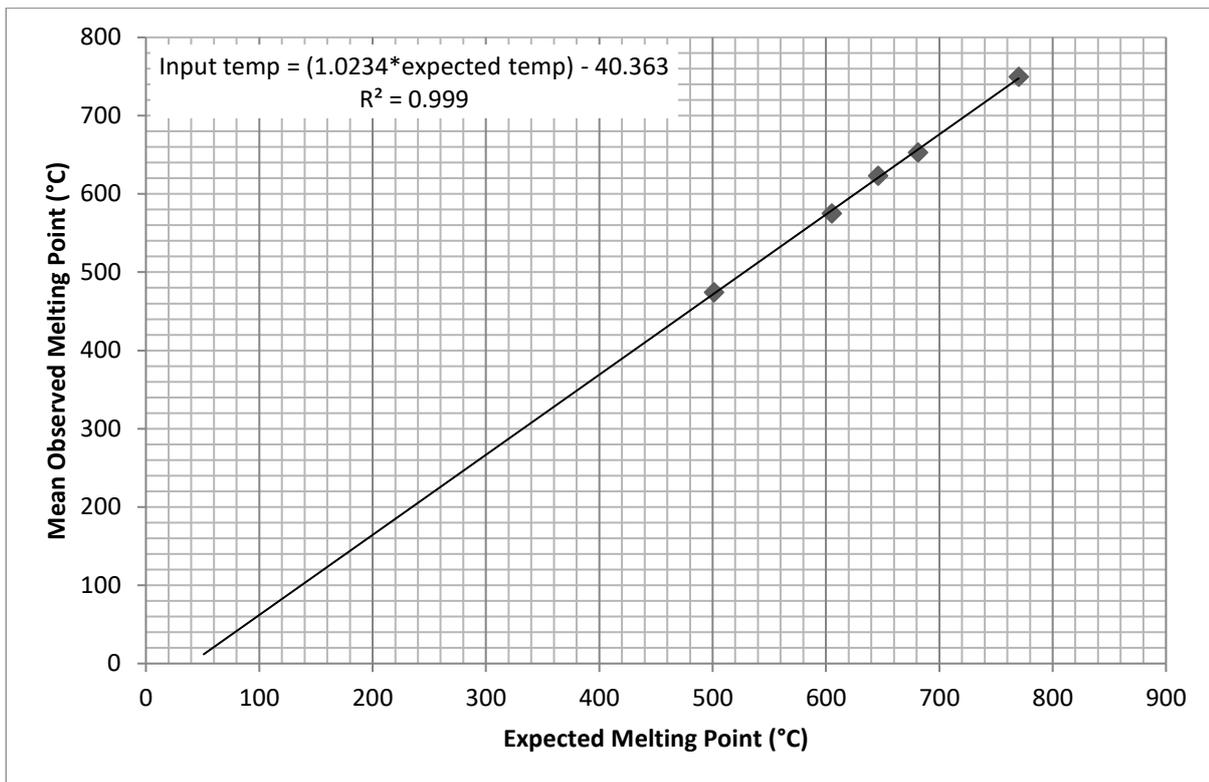
Fig. 2.7. Temperature calibration of pyroprobe.
