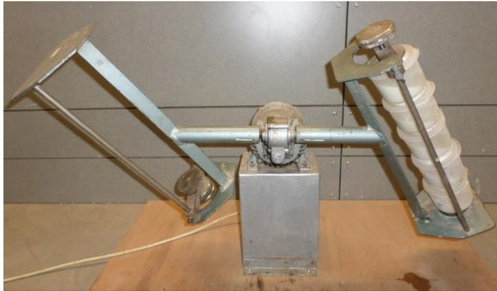
**Figure 3.2:** End-over-end bottle shaker.
