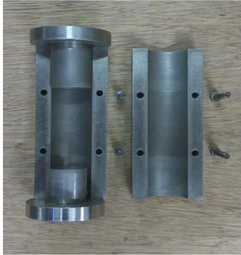
**Figure 3.8:** Split specimen mould.
