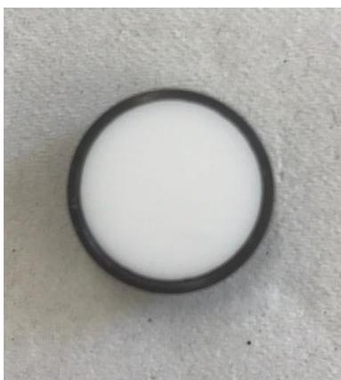
*Figure 2.14. Photograph of Macor disc in the sample cup.*
