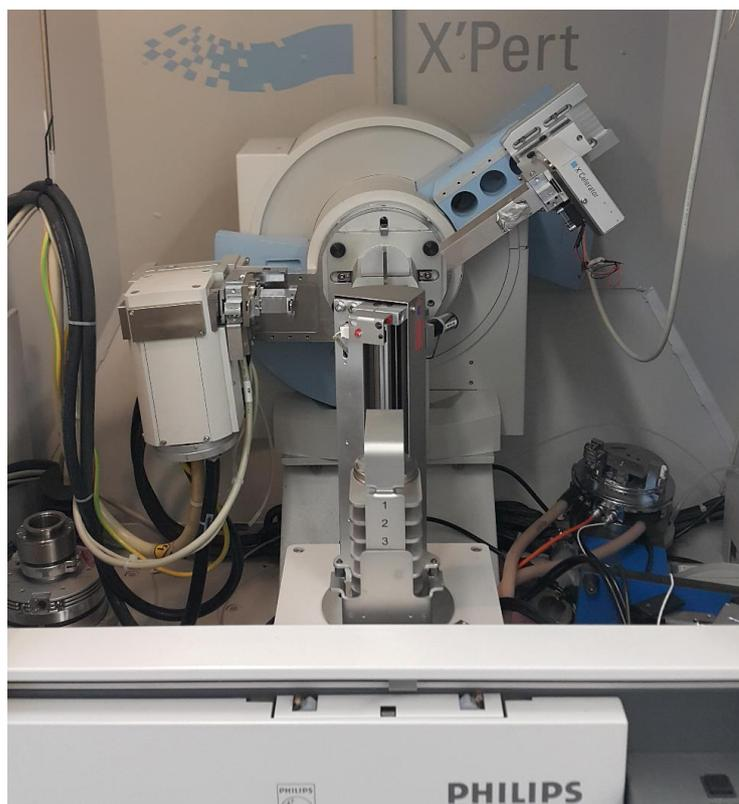
*Figure 2.18. Photograph of the PANalytical X'Pert Pro MPD x-Ray diffractometer.*
