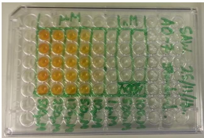
**Figure 2.3 An AO-7 standard curve plated into 96-well plate format**
