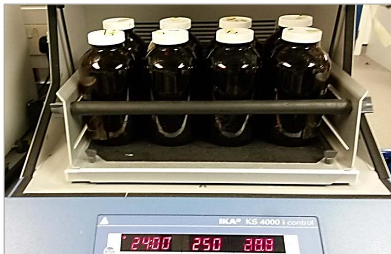
Figure 6.5. Batch reactors for optimisation of estrogen removal via adsorption process. The 500 ml samples contained  $200 \text{ ng.L}^{-1}$  of estrone in synthetic wastewater.
