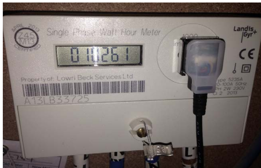
Figure 3.10 T7311 LED lamp pulse sensor with the electricity meter.
