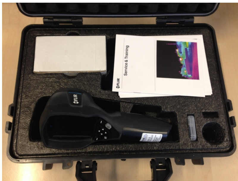
Figure 3.3 FLIR i7 thermal imaging camera.
