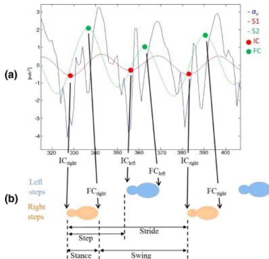
Figure 3: Derived temporal gait measures (step time, stride time, stance time, swing time). Figures adapted from Validation of an accelerometer to quantify a comprehensive battery of gait characteristics in healthy older adults and Parkinson's disease: toward clinical and at home use. By S Del Din, A Godfrey, L Rochester. "IEEE J Biomedical Health Informatics", Volume 20, Issue 3 page number 2168-2194. © 2015 Published by IEEE (Del Din *et al.*, 2015).
