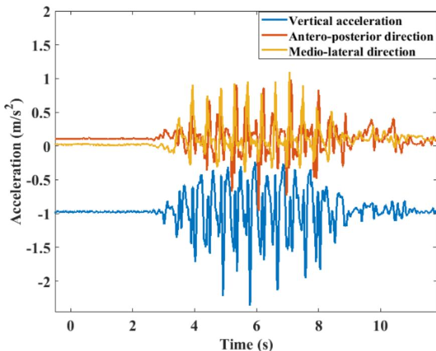
Figure 1: Raw acceleration signal obtained from BWM during the intermittent fast walk test: Orange lines is the acceleration measured in AP direction, yellow lines in ML direction and blue lines in vertical direction.
