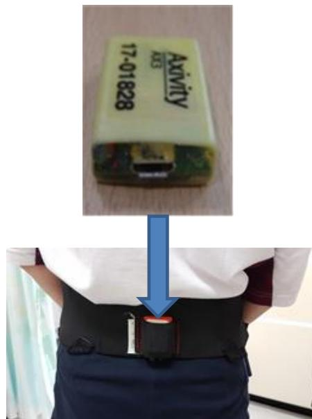
Figure 6-5: BWM on low back at fifth lumbar vertebra, (L5) level for laboratory testing
