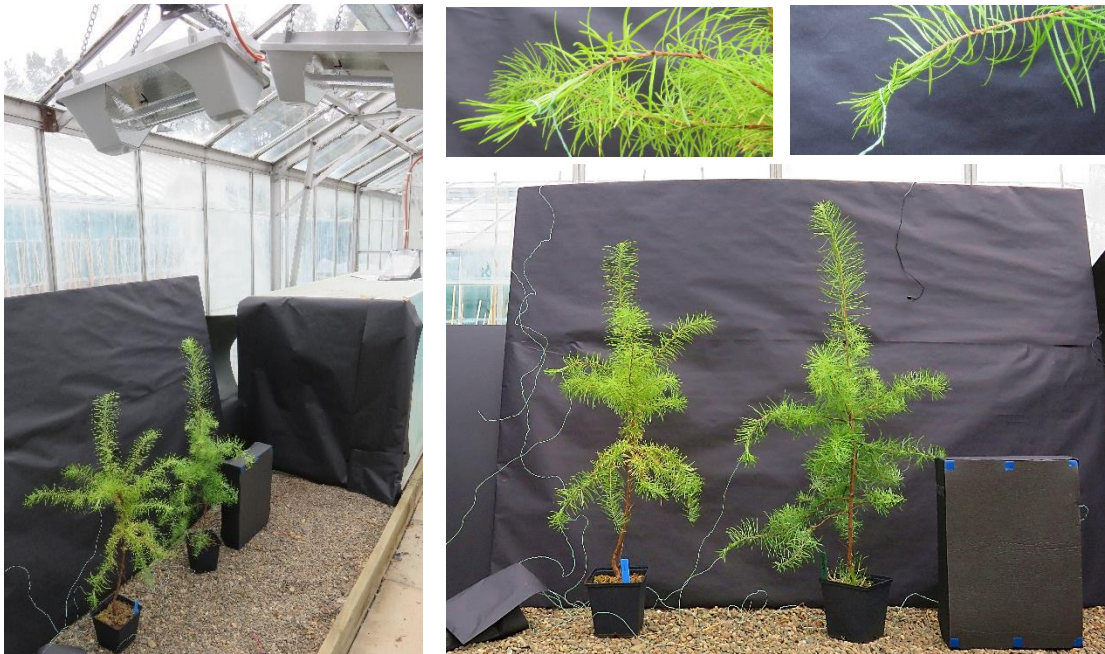
Figure 5.1: Experiment 1 set-up with calibration target on the right; thermocouples were wrapped inside of needle clumps, as shown on the insets.
