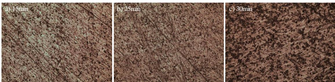
Figure 5.5: Aluminium surfaces after: a) 15min, b) 25min and c) 30min of anodising (OM - 10x).
