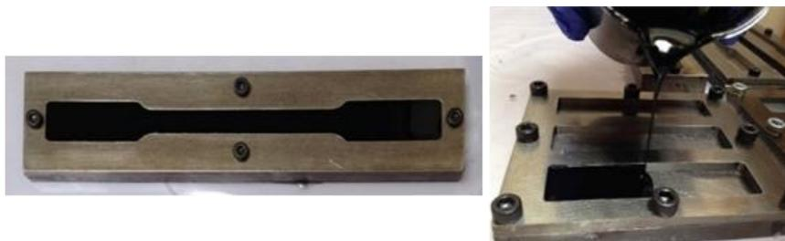
Figure 4.6: Casting process: tensile test mould (left) and flexural test mould (right).
