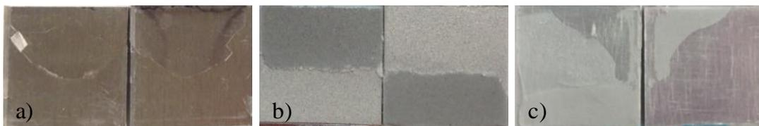
Figure 5.19: Bonding area of Aluminium/Aluminium single lap joints after failure: a) no surface preparation, b) grit blasting and c) etching-anodising.
