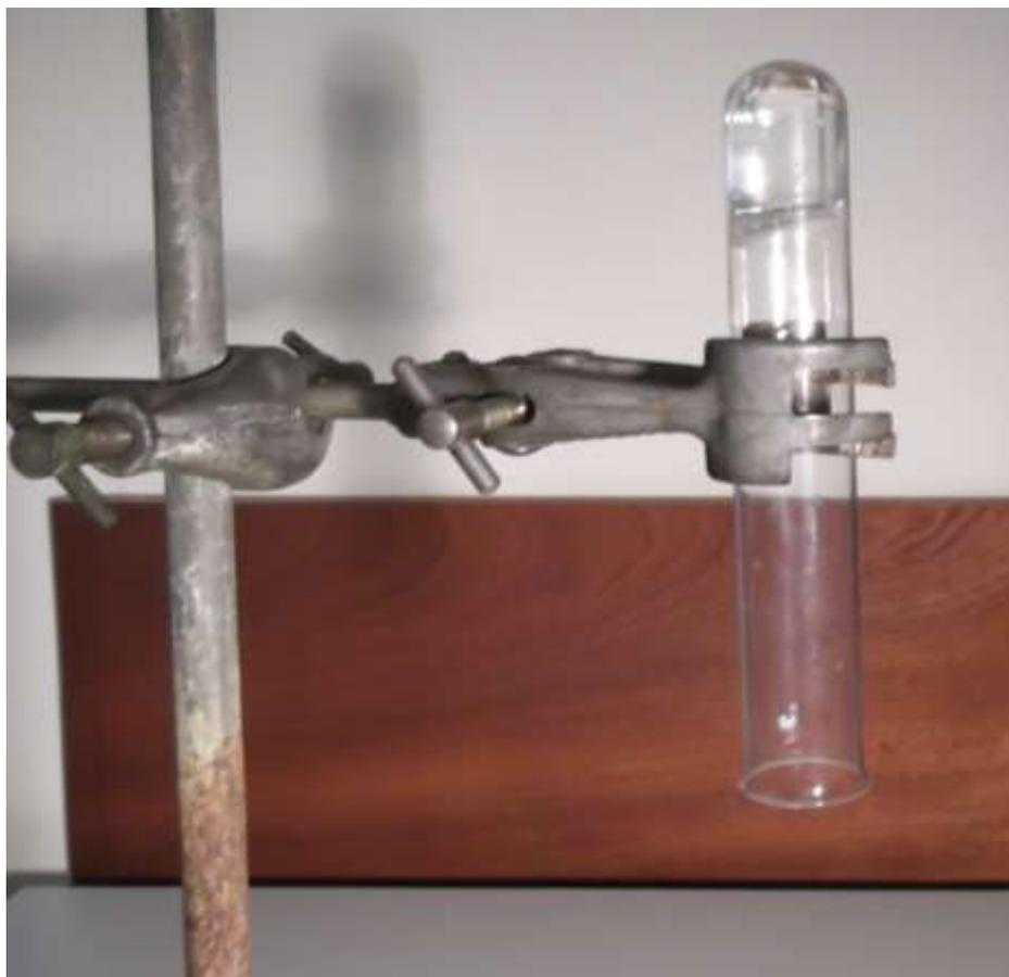
**Figure 8.22** – PMMA photo-polymerised in the presence of P2B which itself is bleached to leave a clear solid. Conditions were not optimised.
