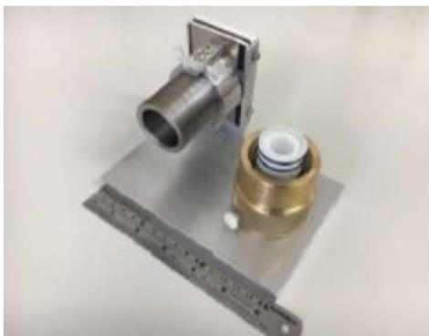
**Figure 2.2** – Variable path length cell used to measure high concentrations or alternatively long path lengths.
