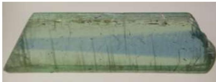
**Figure 5.1** – A microtomed slice of the mineral Kyanite, the green colour originates from ferric ions while the blue band is due to an IVCT transition between  $Fe^{2+}$  and  $Fe^{3+}$ .
