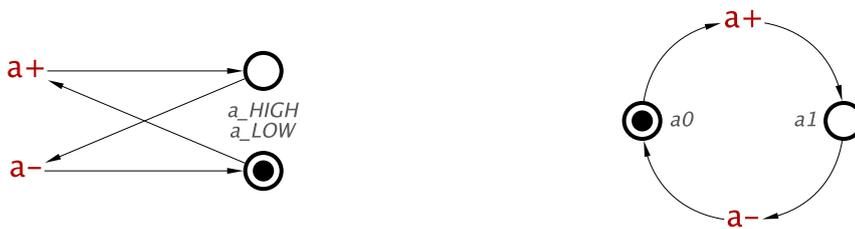
(a) "Z" formation of a signal transition loop      (b) "Loop" formation of a signal transition loop
