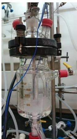
Figure 3-2 Amidation kinetic study in a 150 mL stirred tank reactor
