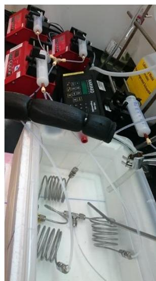
Figure 4-3 (a) Setup of the stainless steel reactor; (b) Reagents delivered into stainless steel reactor via syringe pumps, submerged in circulated silicone oil bath.
