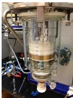
Figure 3-1 Base case amidation reaction in a 500 mL RC 1 reactor.
