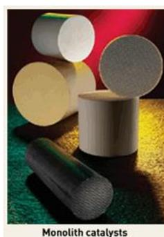
Figure 2-14 Example of monoliths (Rouhi, 2003)
