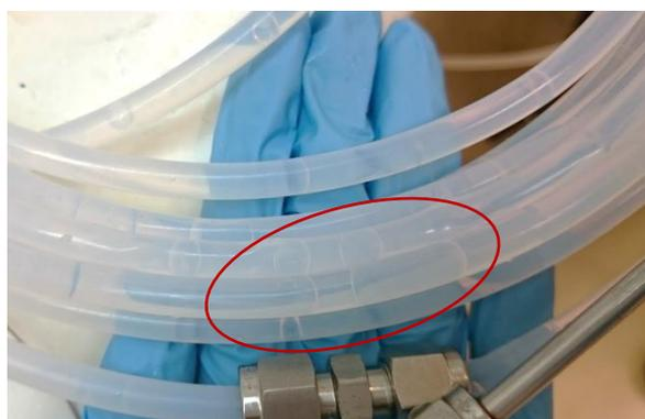
Figure 3-13 Photo of large biphasic slugs of toluene and water phases in the bare PTFE tubing section. Large liquid-liquid slugs observed in red circle
