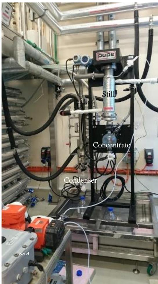
Figure 3-7 POPE Wiped Film Evaporator used in actual experiments.
