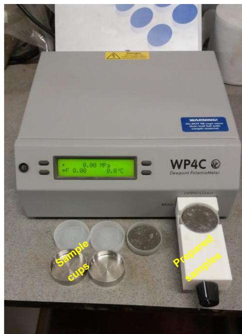
Figure 3.18: Dew point potentiometer with soil specimen for measurement of suction
