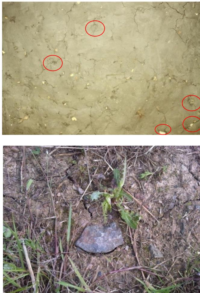
Figure 4.27: Cracking around location of flaws in the soil (top photo) Laboratory (bottom photo) Field
