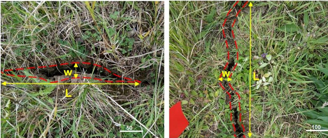
Figure 5.36: Surface crack geometry. Crack length, **L** is  $\gg$  width, **W**.
