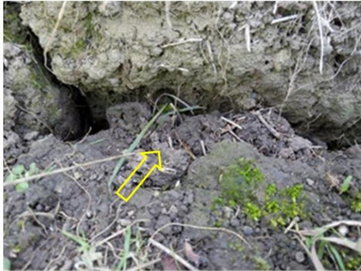
Figure 5.32: Loose and wetted soil particles (arrowed) swells within a crack. The fallen soil particles either directly filled up the crack by mass or swell in volume and fill the cracks when wetted. The process of crack closure through filling and swelling of expansive soil particles is illustrated in Figure 5.33.
