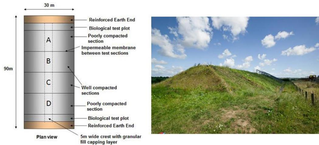
Figure 3.1: Layout and part of physical structure of the embankment. adapted from (Hughes *et al.*, 2009; Toll *et al.*, 2012)
