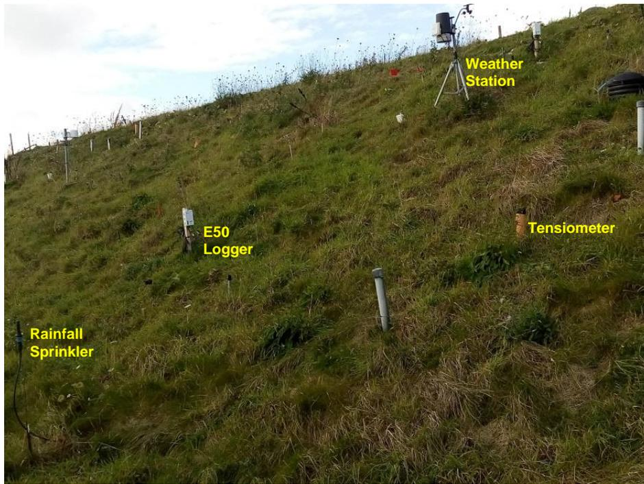
Figure 3.2: Some of the monitoring instrument on a section of the embankment
