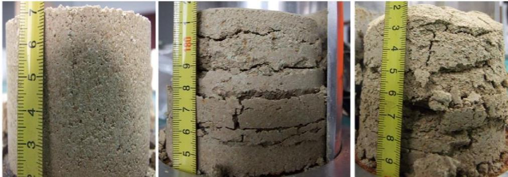
Figure 2.26: Homogenous to aggregated structure (Left to right) and volume change in a soil after 3 wet-dry cycles. From (Tang *et al.*, 2016).
