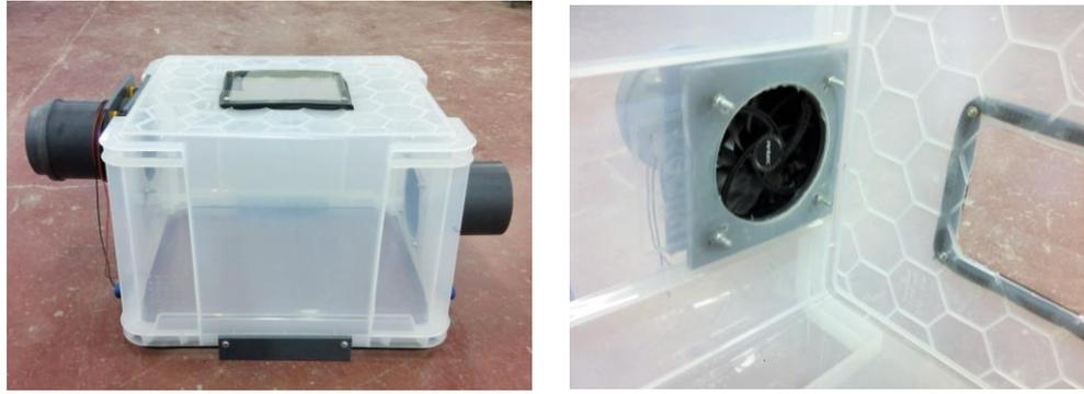
Figure 3.13: The climate cover fitted with axial fan
