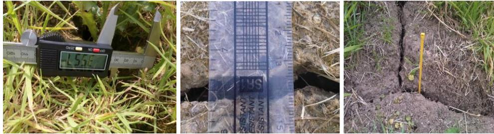
Figure 3.6: Line gauges and probes for crack geometric measurement
