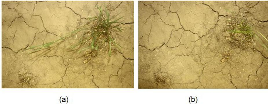
Figure 5.19: Crack pattern in experimental rooted soil (a) 1<sup>st</sup> cycle (b) 2<sup>nd</sup> cycle
