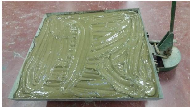
Figure 3.17: Bentonite-Nafferton clay mixture undergoing drying processes
