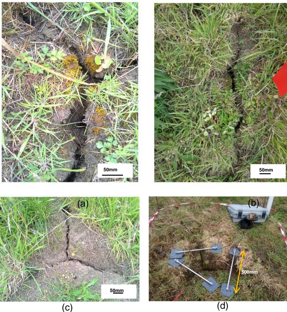
Figure 4.14: Surface cracks in the embankment and displacement monitor installed in one of the cracks location (d).
