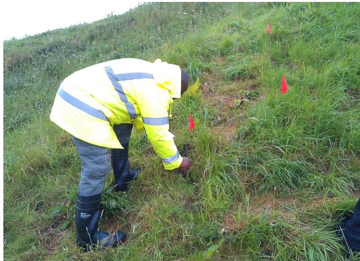
Figure 3.5: Crack survey on Bionics embankment. Crack location marked with red flags
