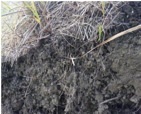
Figure 5.17: Fibrous grass roots in a test pit section on the embankment
