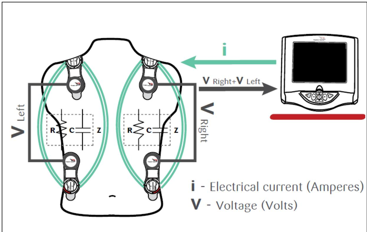
The monitor induces an electrical current (labelled with  $i$ ) with a frequency of 75KHz. The returning voltage is detected on both sides (labelled as  $V$ ). The monitor measures the time delay between  $i$  and  $v$ , thus detecting the phase shifts. (Reproduced from Cheetah Medical<sup>®</sup>)
