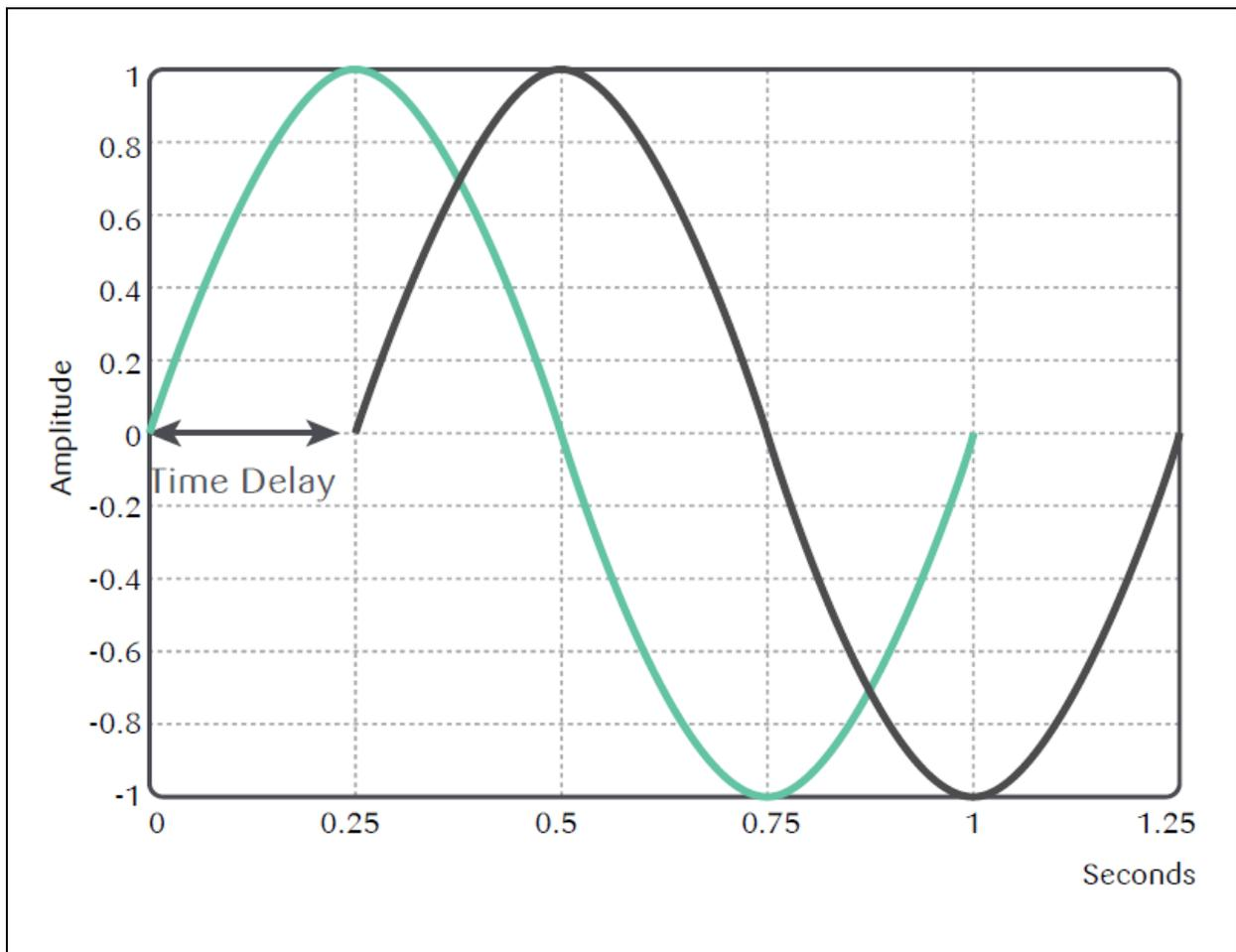
The AC is based on the sine wave. Therefore, the green sine wave starts 0.25seconds before the black sine wave. The black sine wave is phase shifted by  $90^\circ$  or quarter of cycle from the green sine wave. This angle can be used to calculate the stroke volume. (Reproduced from Cheetah Medical®)
