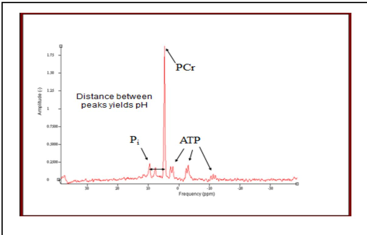
MR signal can detect peaks of PCr, P<sub>i</sub> and three peaks of ATP ( $\gamma$ ,  $\alpha$  and  $\beta$  in that order). The gap between PCr and P<sub>i</sub> can be used to calculate the pH. (Figure from Dr K Hollingsworth)
