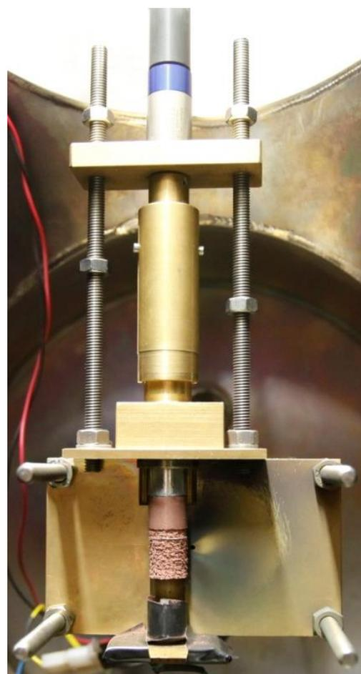
Figure 3.5 Schematic of ablation source B, alongside a photograph of the source inside the Newcastle CP-FTMW spectrometer.
