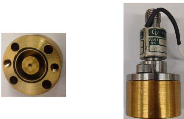
Figure 3.6 (Left): Photograph of the water reservoir used in this work. (Right): Photograph of the assembled nozzle and reservoir.
