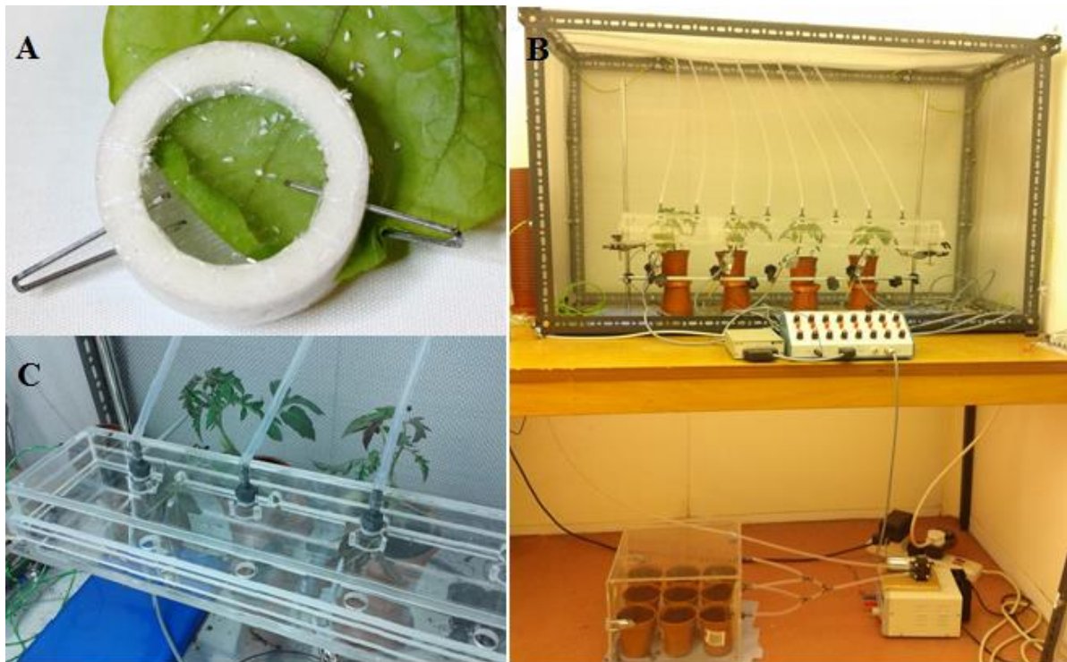
Figure 2.2: (A) Clip cage used in no choice and video trials. (B) EPG equipment used for EPG studies. (C) Detail of volatile delivery box and positioning of plants for EPG studies.
