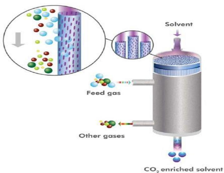
Figure 2.3: The schematic diagram of membrane gas absorption.
