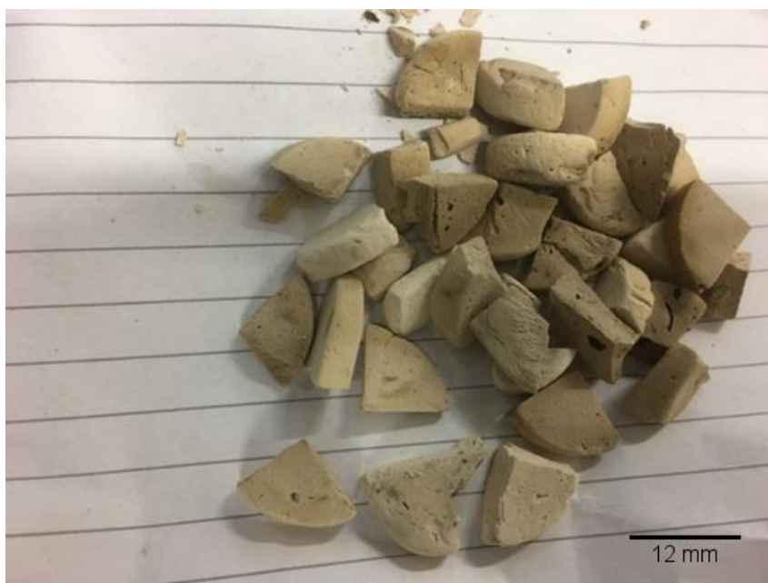
Figure 3-6. The PolyHIPE beads after sulphonation process
