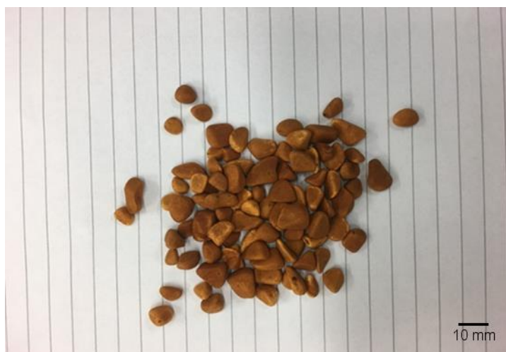
Figure 3-8. PolyHIPE beads after coating with iron oxide
