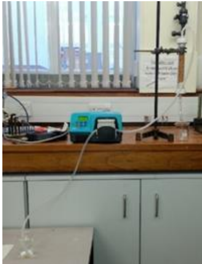
Figure 3-22. The cyclic filtration process
