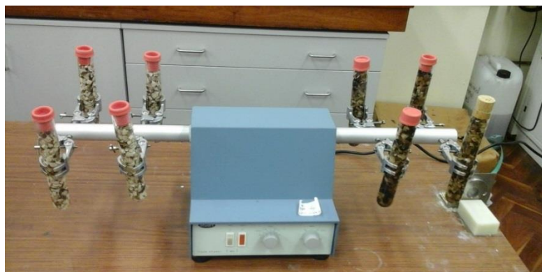
Figure 3-23. The filtration processes with shaking
