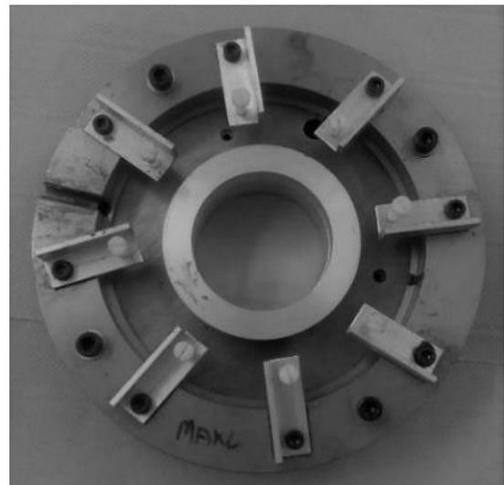
(b) Slot components assembly mould
