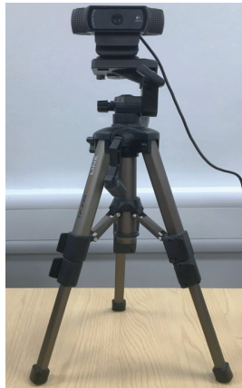
Figure 5.11: The Logitech HD c920 webcam setup which is fixed on a tripod for real-time image acquisition.
